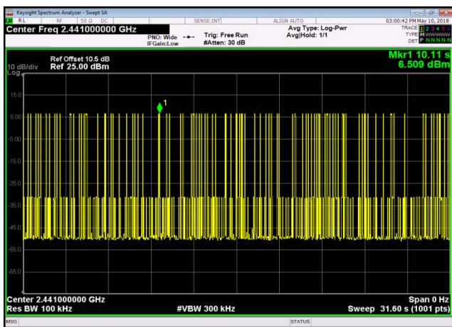
Dwell Time: GFSK,2480,DH5,Transmission Number
