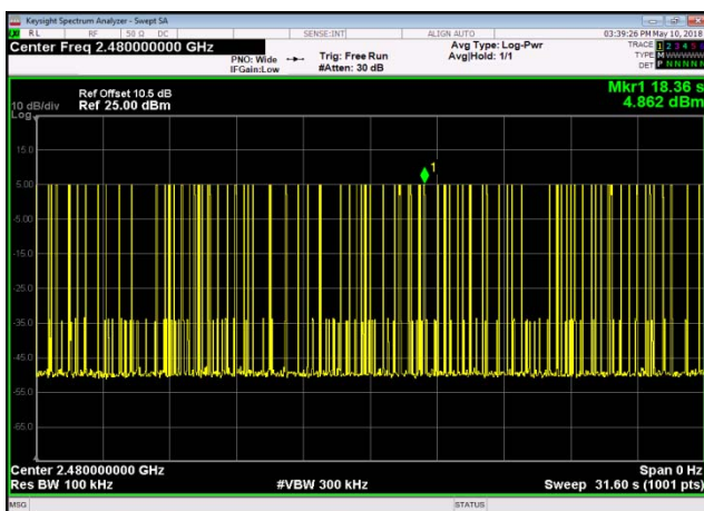
Dwell Time: GFSK,2402,DH5,Transmission Number
