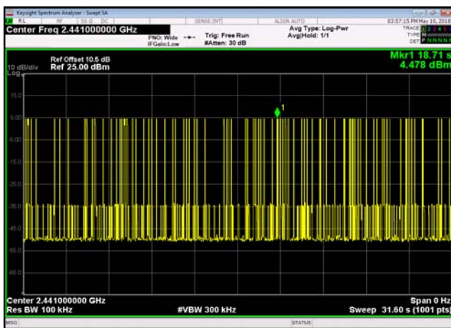
Dwell Time: PI/4DQPSK,2480,2DH5,Transmission Number
