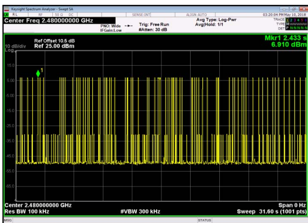
Dwell Time: GFSK,2480,DH5,Transmission Number
