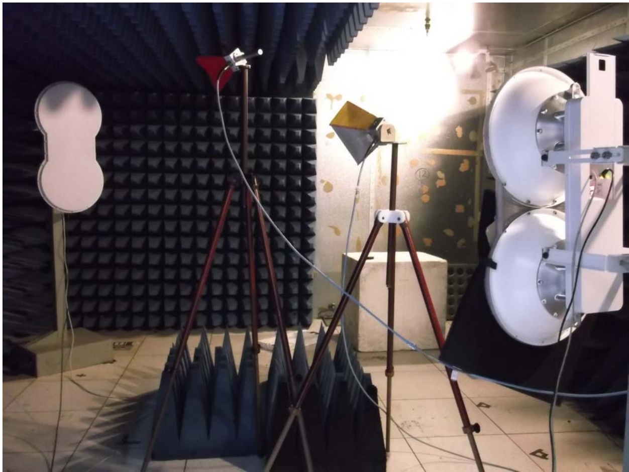
Red antenna (closest to EUT at left) is Radar Transmit Antenna
