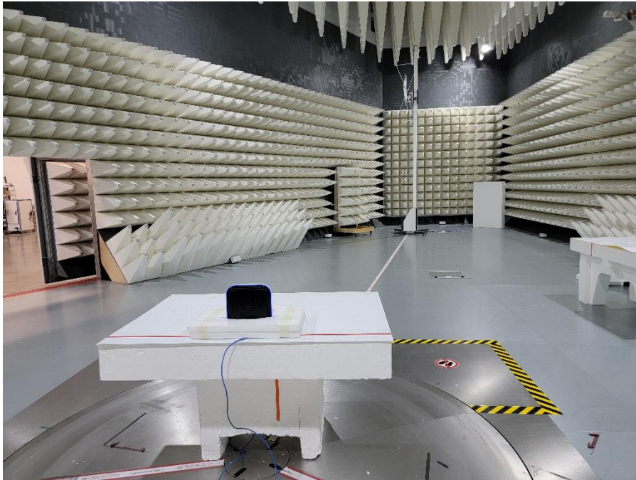
Photograph 1: View Test Set Up Radiated Emissions 30 – 1000 MHz
