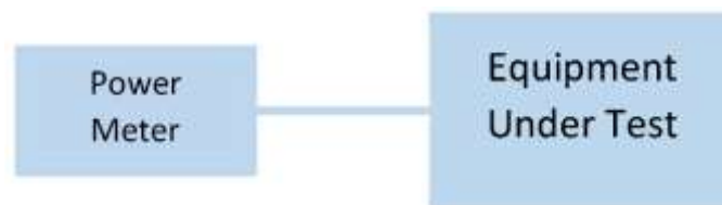
Figure 3: Output Power Measurement
