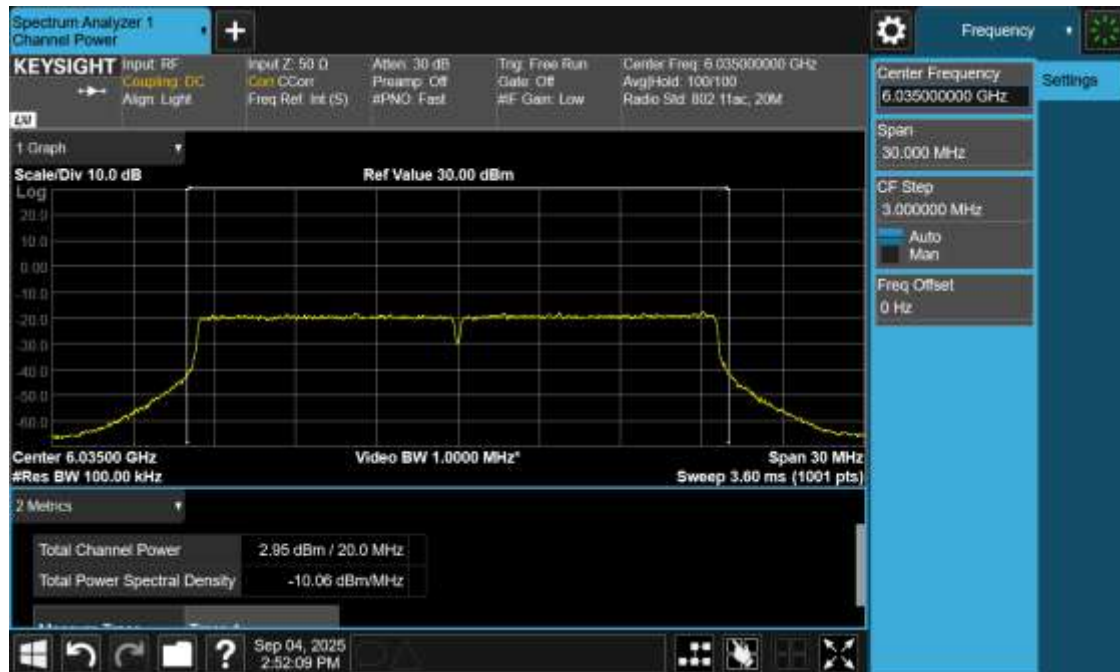
Plot 2: Power and PSD for Standard Power – 6035 MHz
