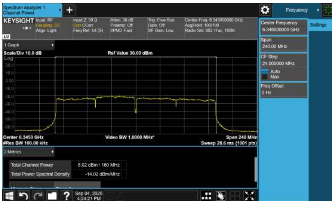
Plot 11: Power and PSD for Standard Power – 6345 MHz
