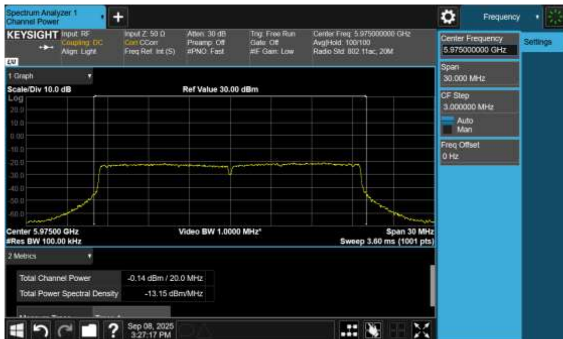
Plot 20: Power and PSD for Low-Power Indoor – 5975 MHz
