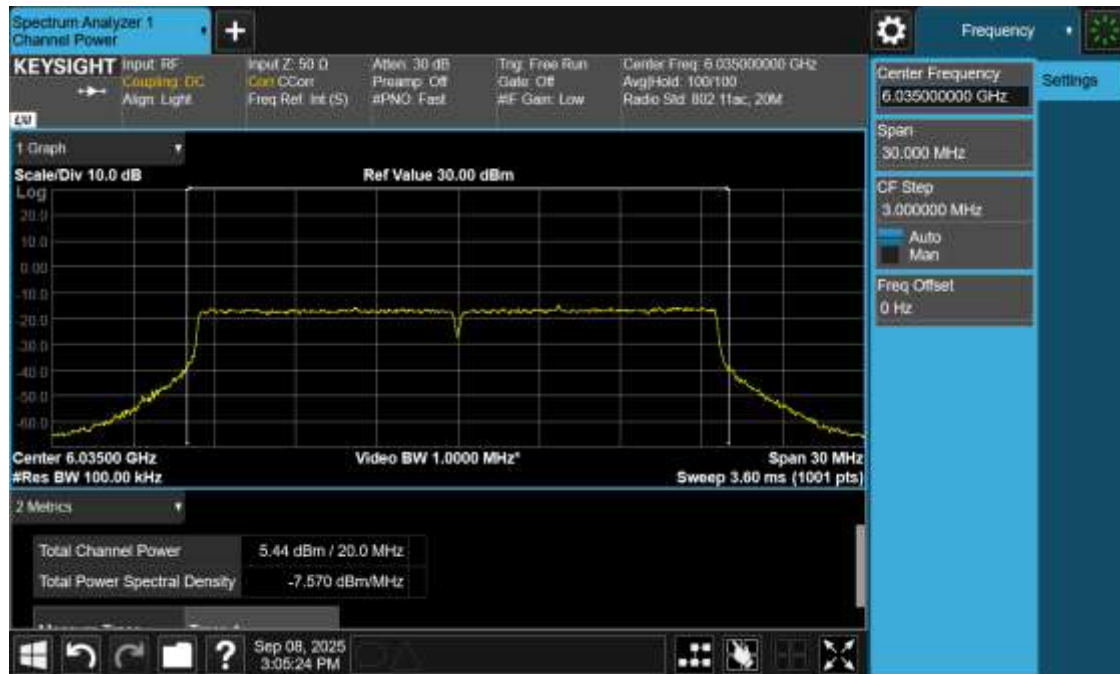
Plot 19: Power and PSD for Standard Power – 6035 MHz
