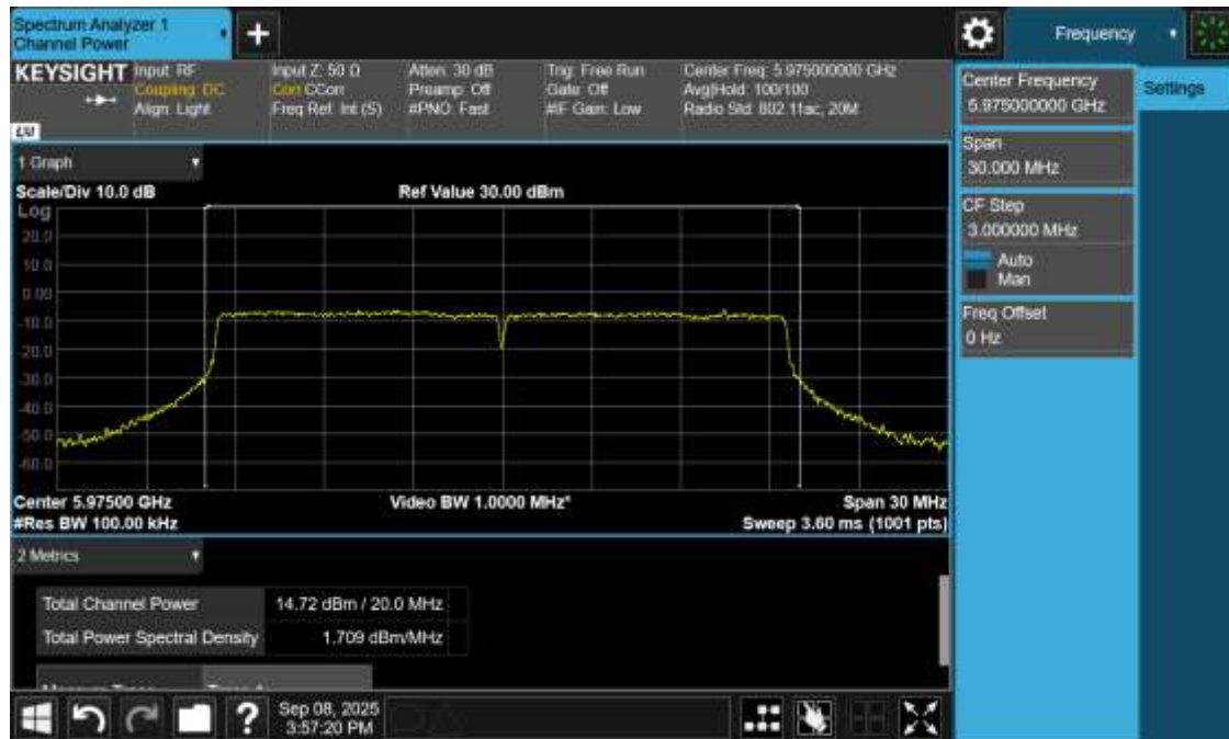
Plot 23: Power and PSD for Standard Power– 5975 MHz
