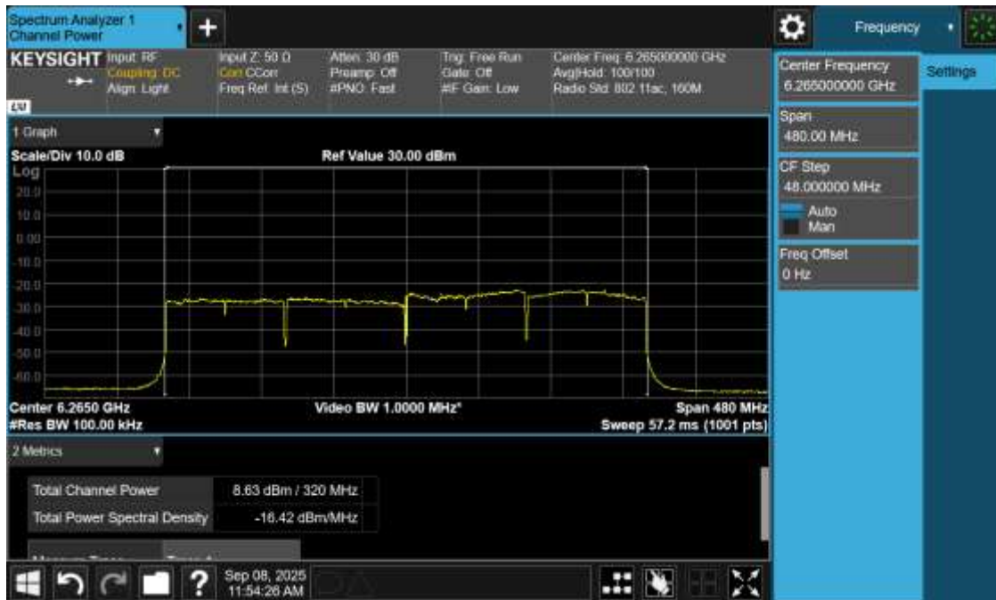
Plot 14: Power and PSD for Standard Power – 6265 MHz
