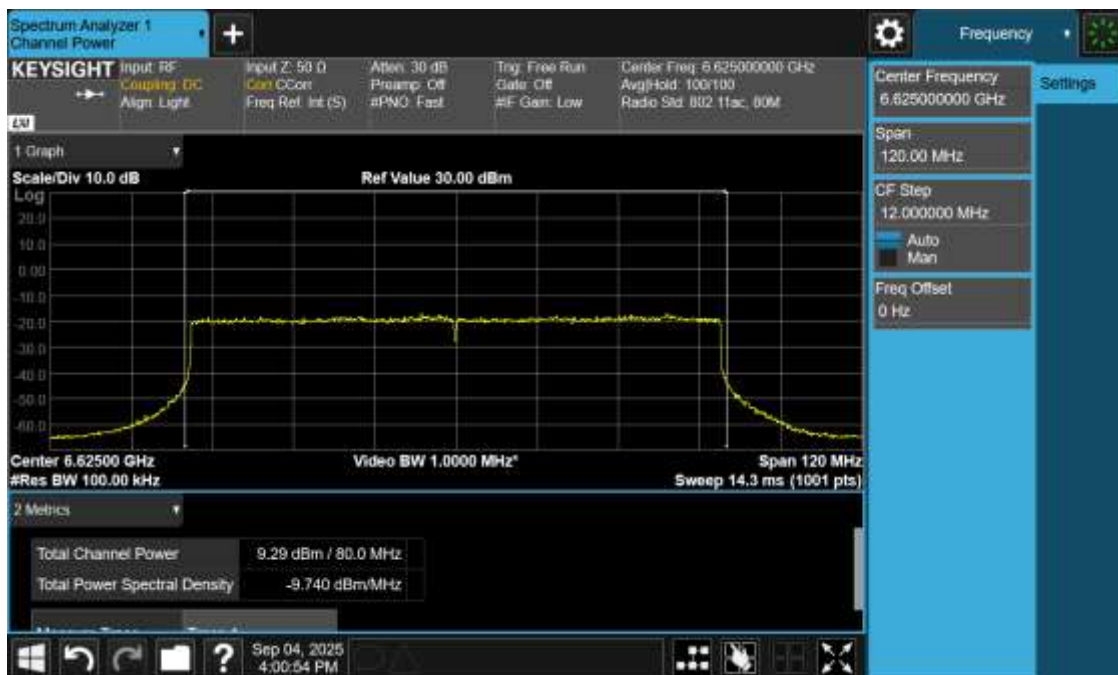
Plot 9: Power and PSD for Standard Power – 6625 MHz
