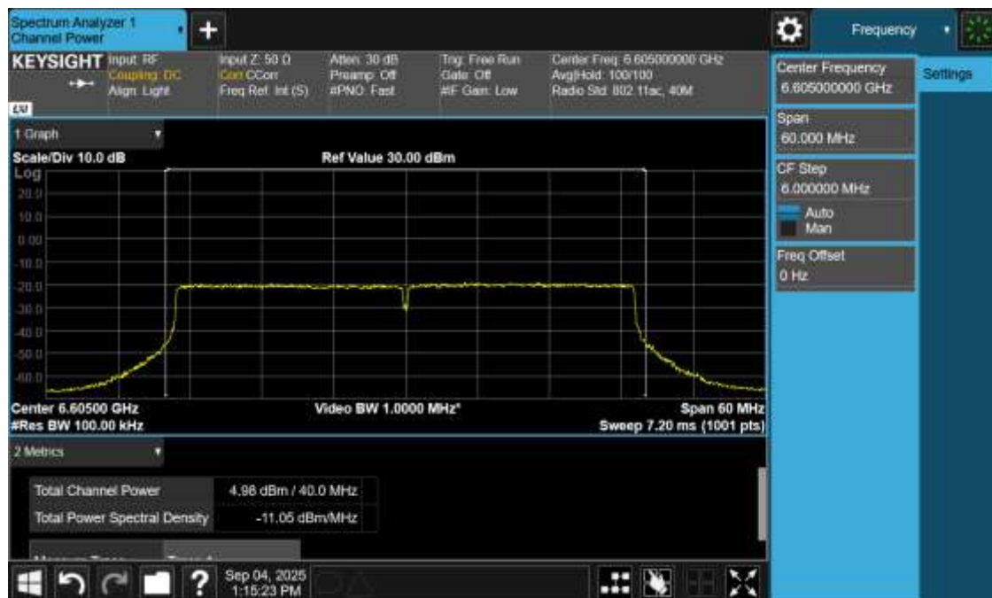
Plot 6: Power and PSD for Standard Power – 6605 MHz
