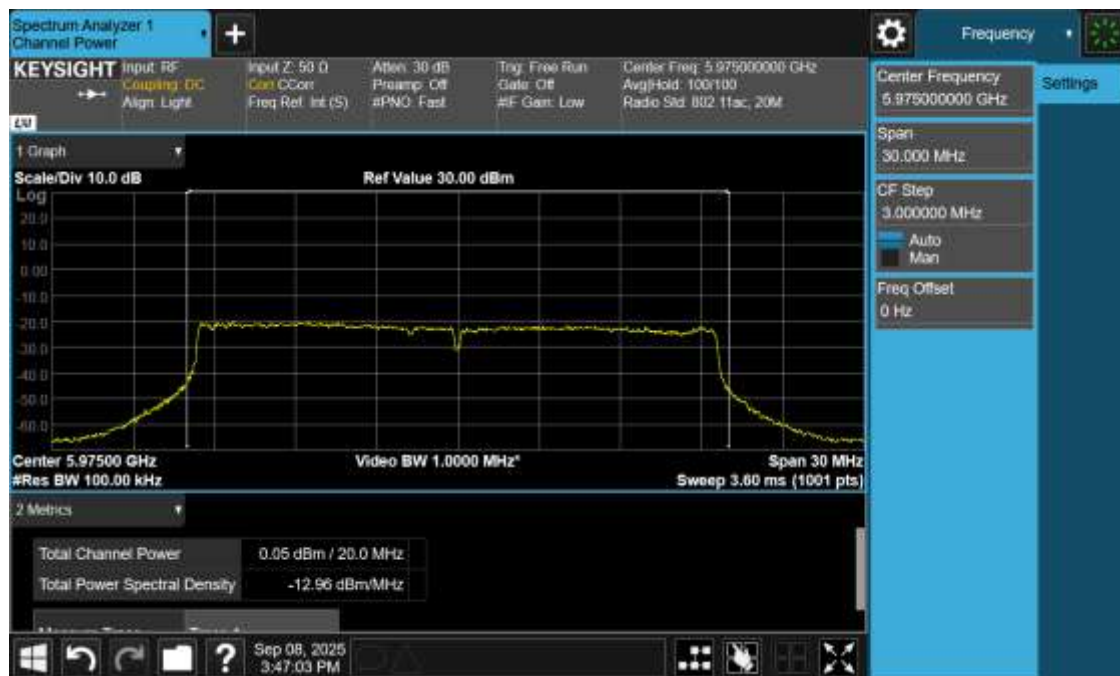
Plot 22: Power and PSD for Low-Power Indoor – 5975 MHz
