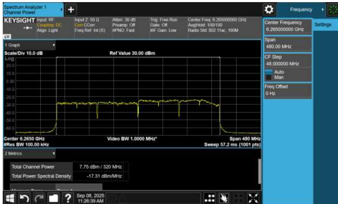
Plot 13: Power and PSD for Low-Power Indoor – 6265 MHz
