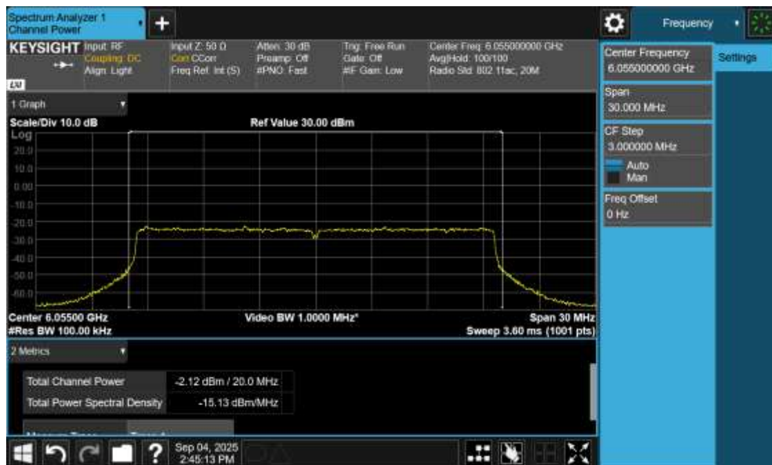
Plot 1: Power and PSD for Low-Power Indoor – 6055 MHz
