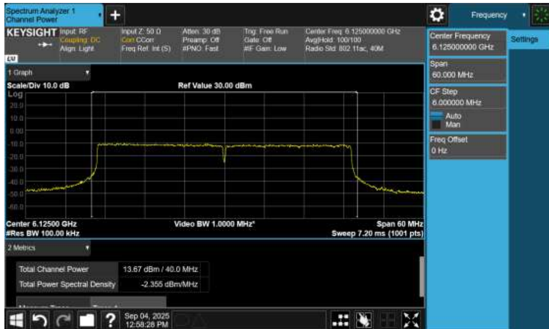
Plot 5: Power and PSD for Standard Power – 6125 MHz
