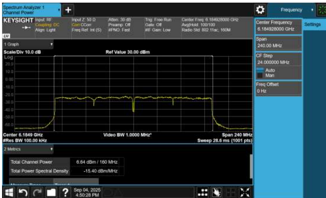
Plot 12: Power and PSD for Standard Power – 6185 MHz
