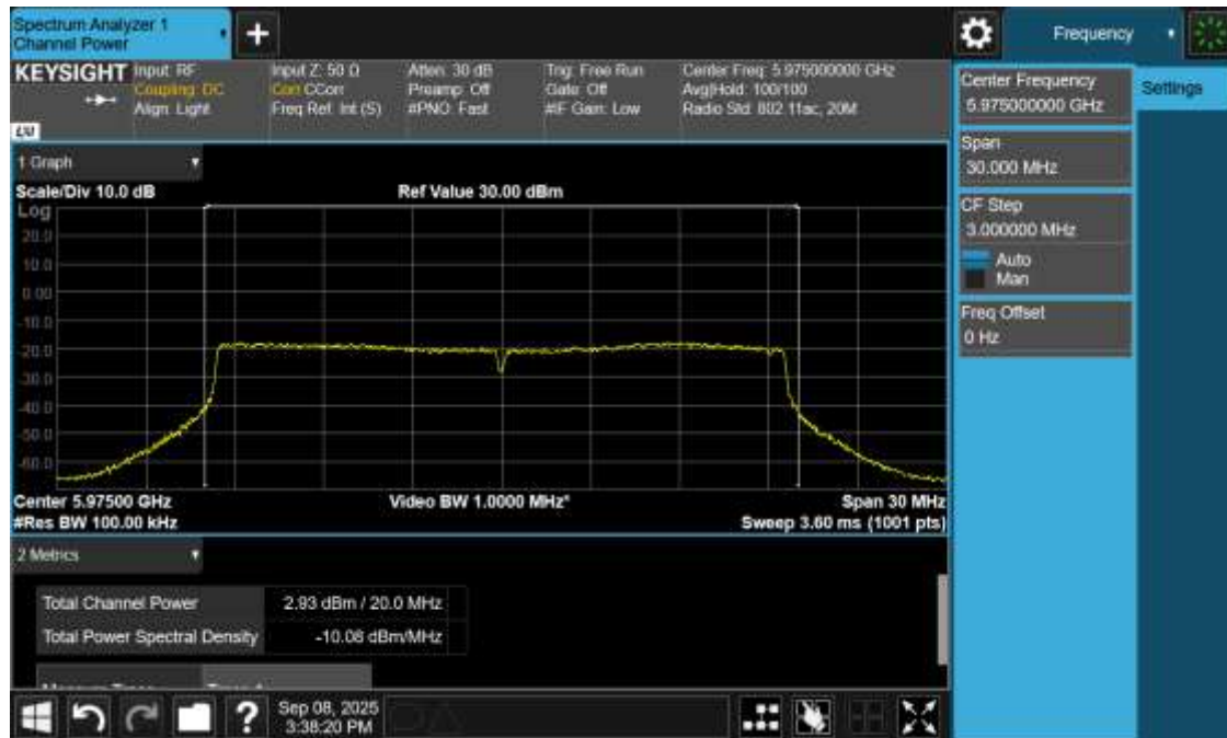
Plot 21: Power and PSD for Standard Power– 5975 MHz
