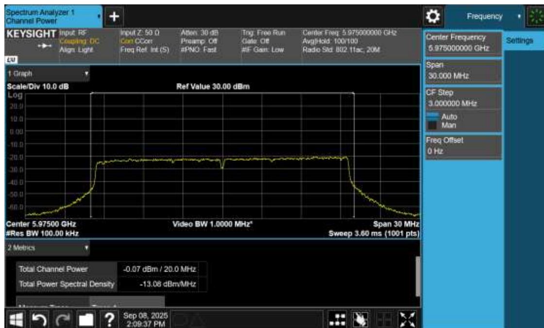
Plot 16: Power and PSD for Low-Power Indoor – 5975 MHz
