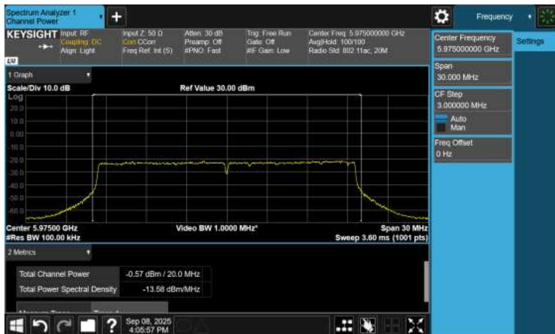
Plot 24: Power and PSD for Low-Power Indoor – 5975 MHz
