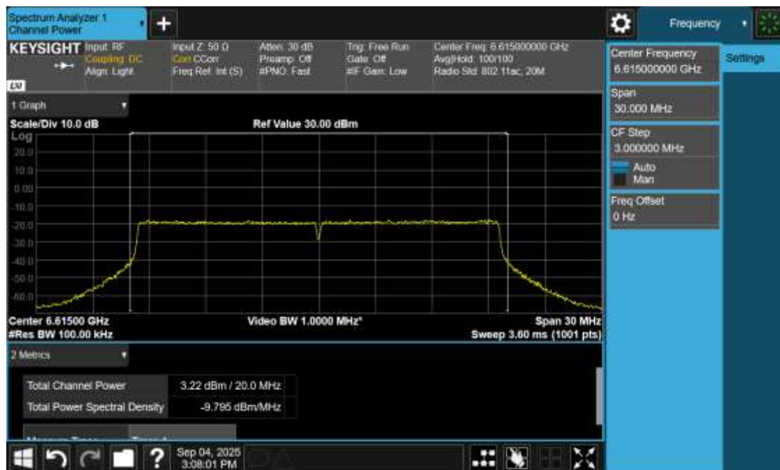
Plot 3: Power and PSD for Standard Power – 6615 MHz
