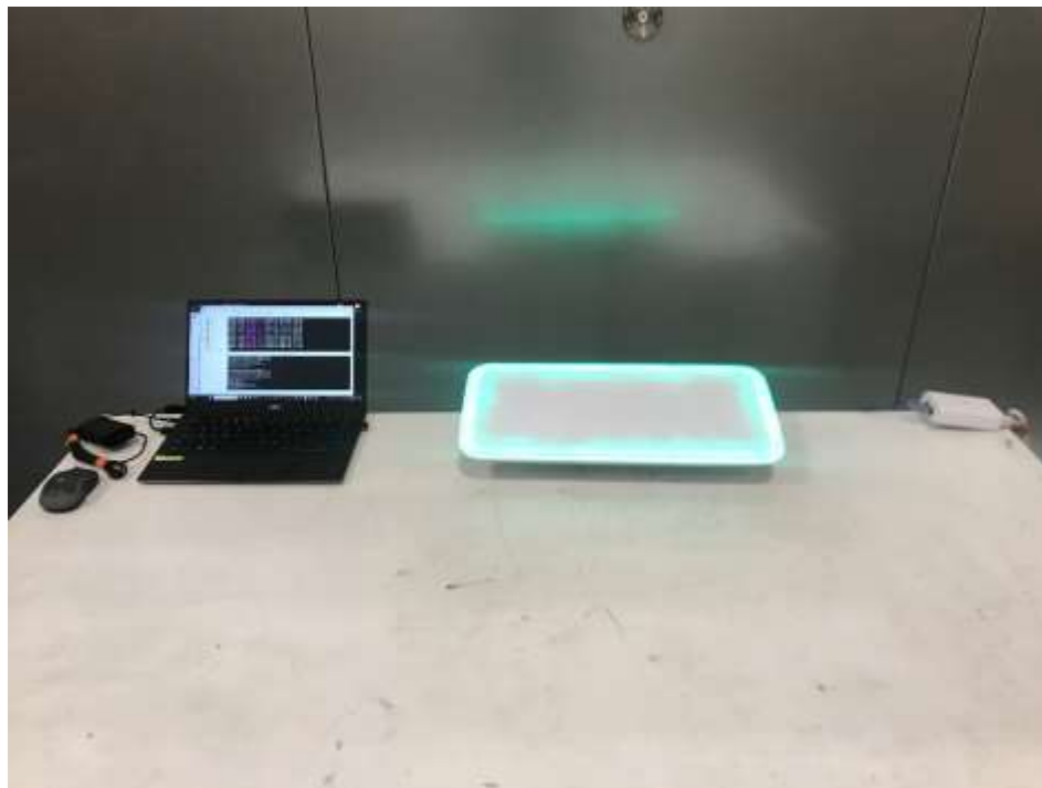
Photograph 7: View Test Set Up Front Conducted Emissions
