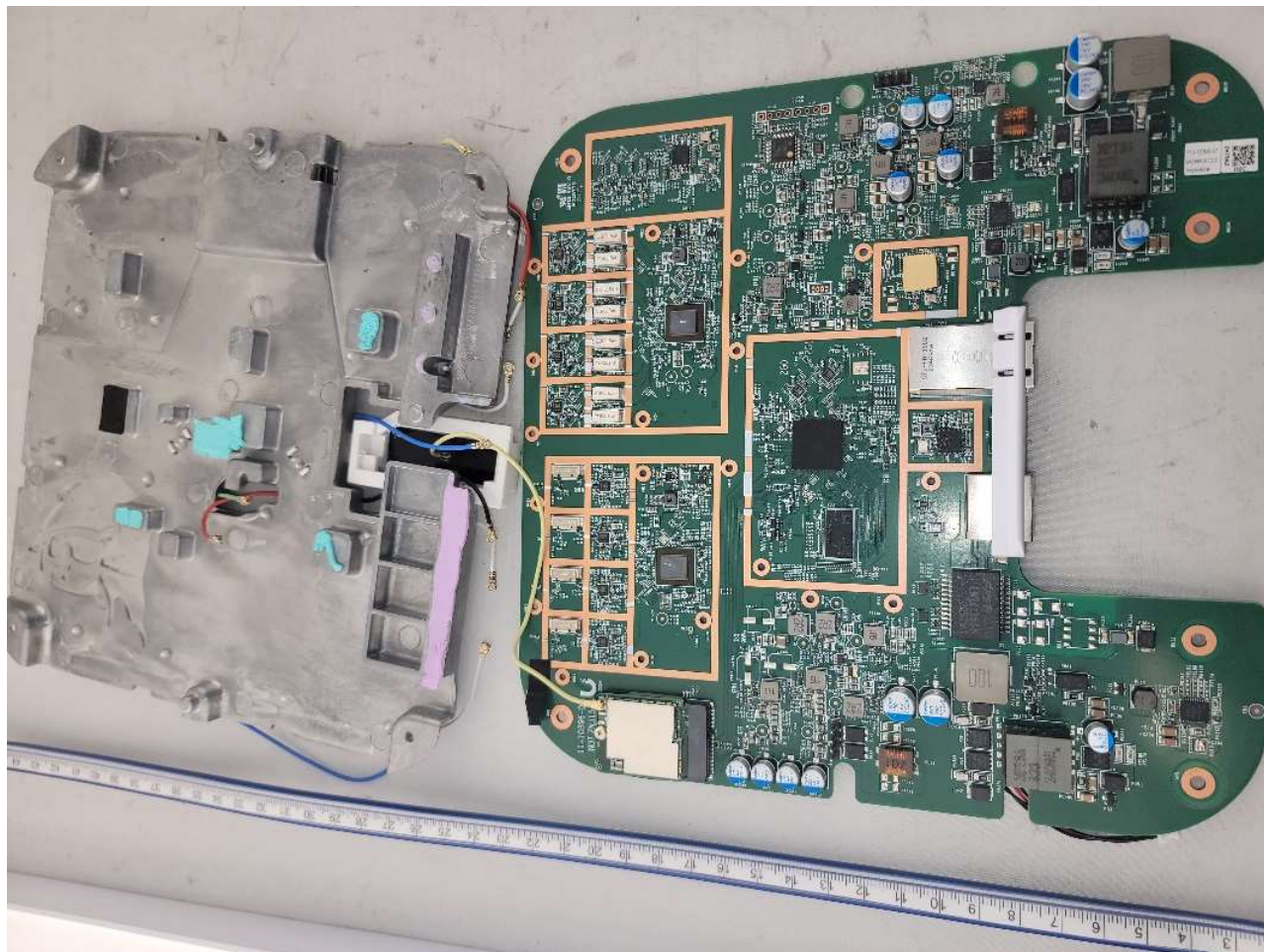
Photograph 4: Antenna Board and PCB Removed From Housing
