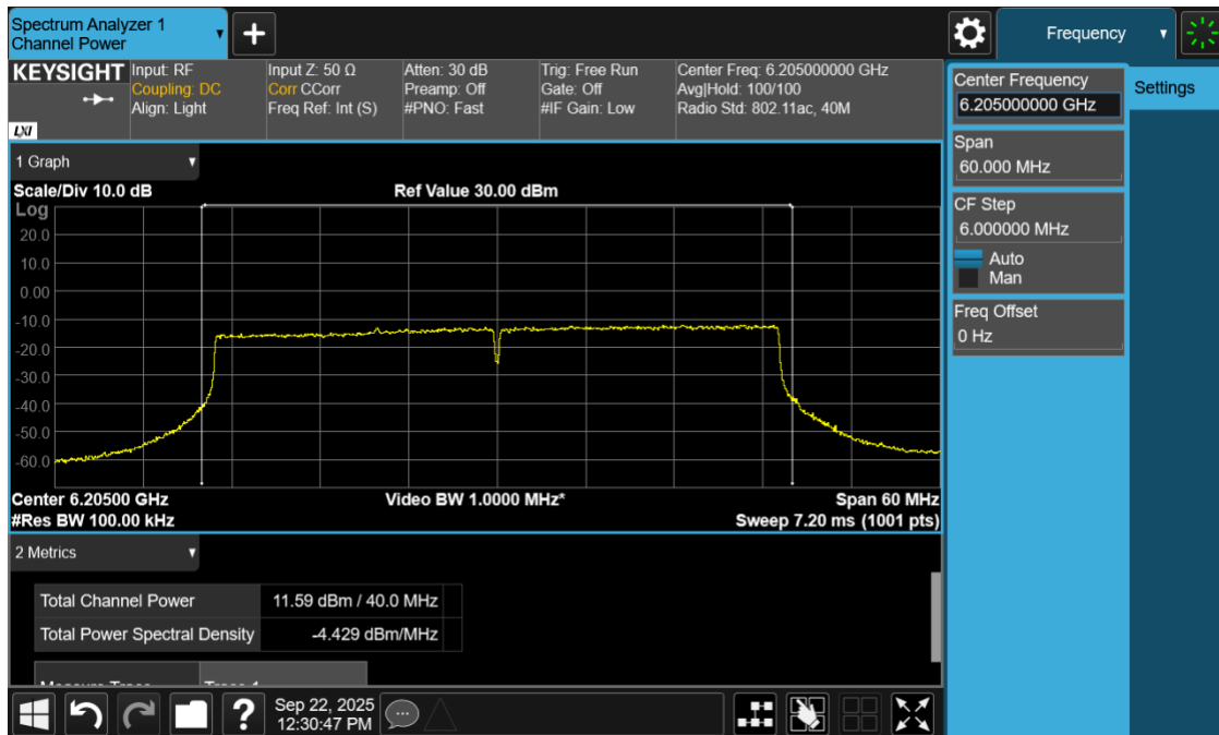
Plot 5: Power and PSD for Standard Power – 6205 MHz
