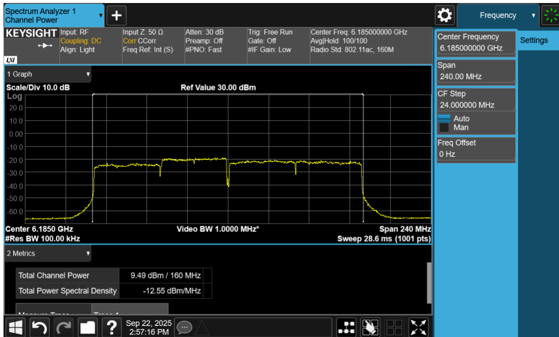
Plot 11: Power and PSD for Standard Power – 6185 MHz
