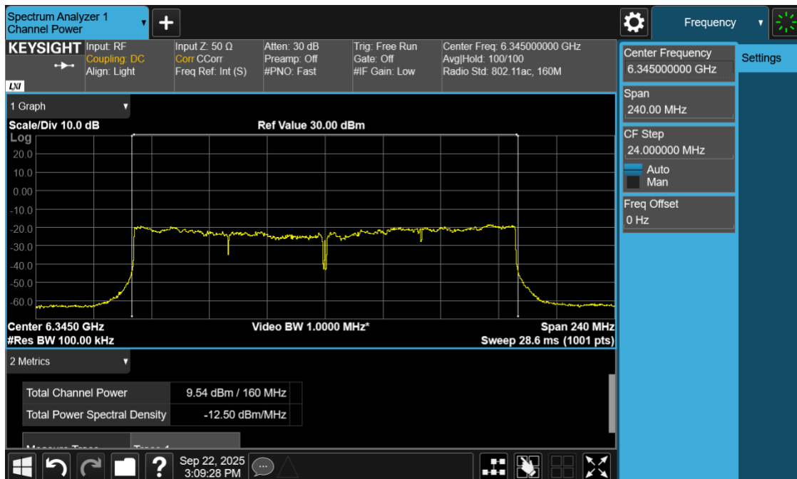
Plot 12: Power and PSD for Standard Power – 6345 MHz
