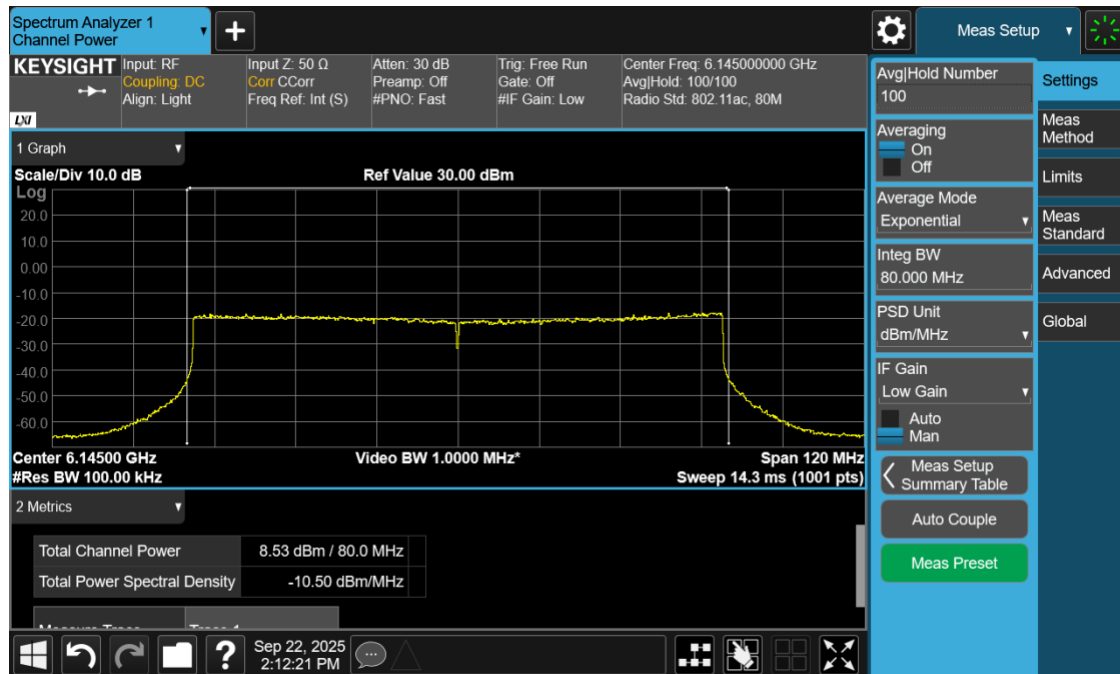
Plot 8: Power and PSD for Standard Power – 6145 MHz
