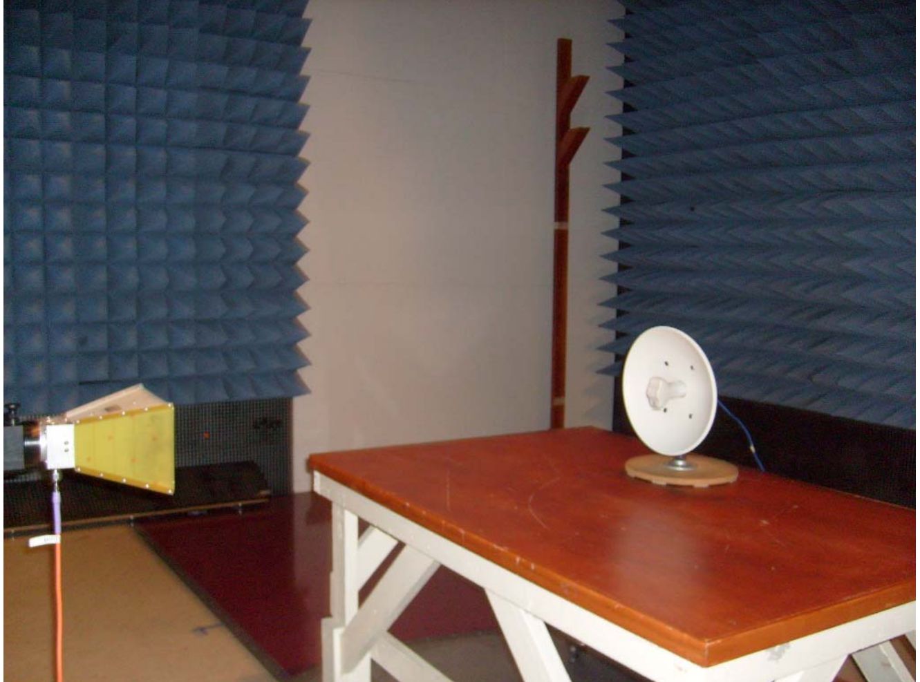
Photograph 5. Radiated Spurious, Test Setup (Dish Antenna)
