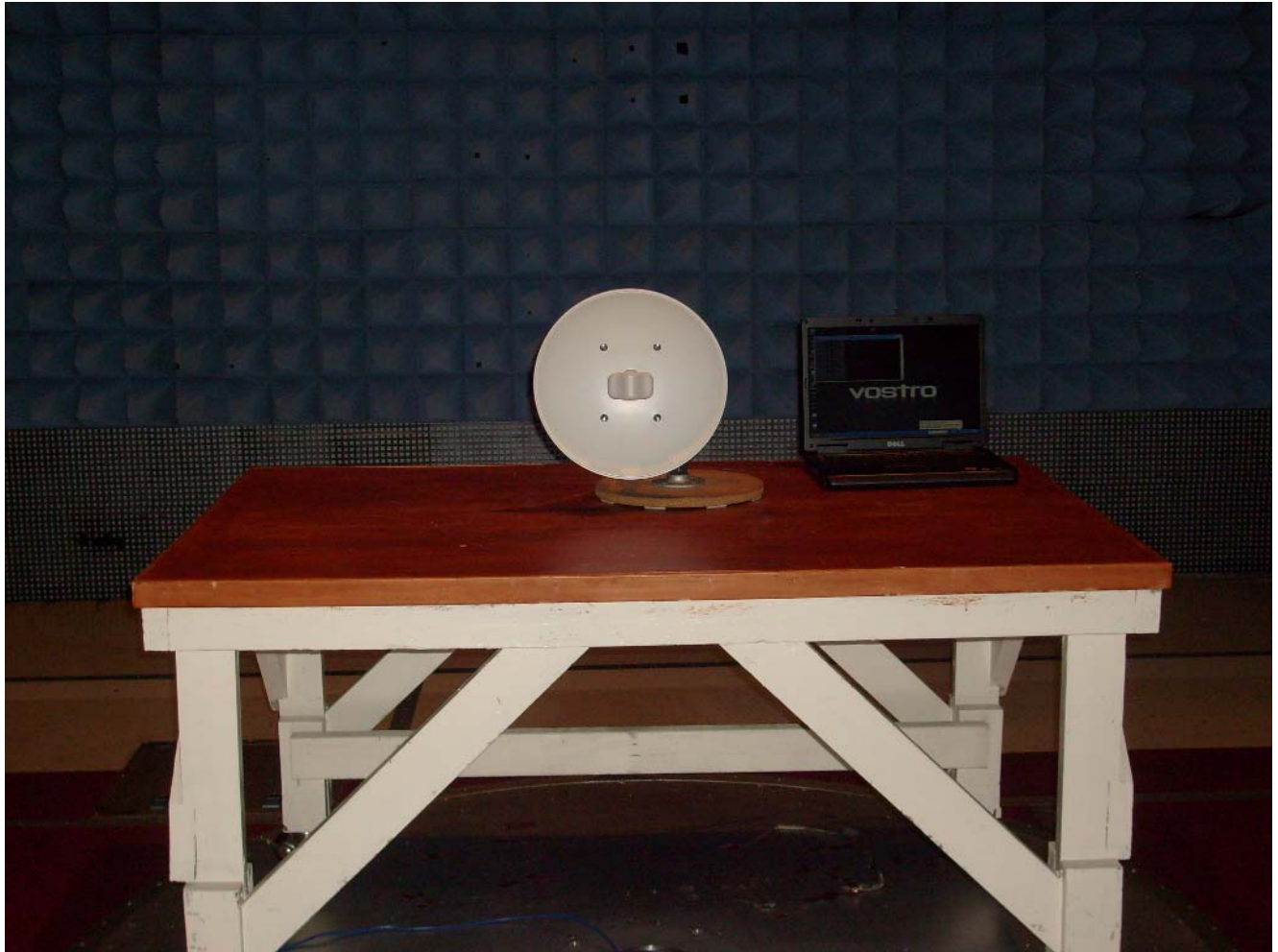
Photograph 2. Radiated Emission, Test Setup
