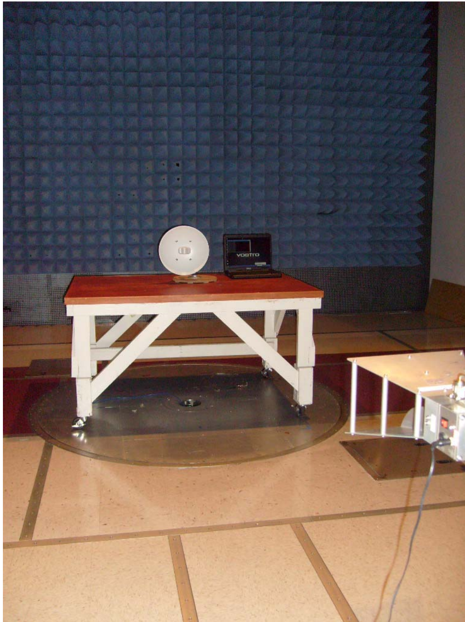
Photograph 3. Radiated Emission, above 1GHz Test Setup
