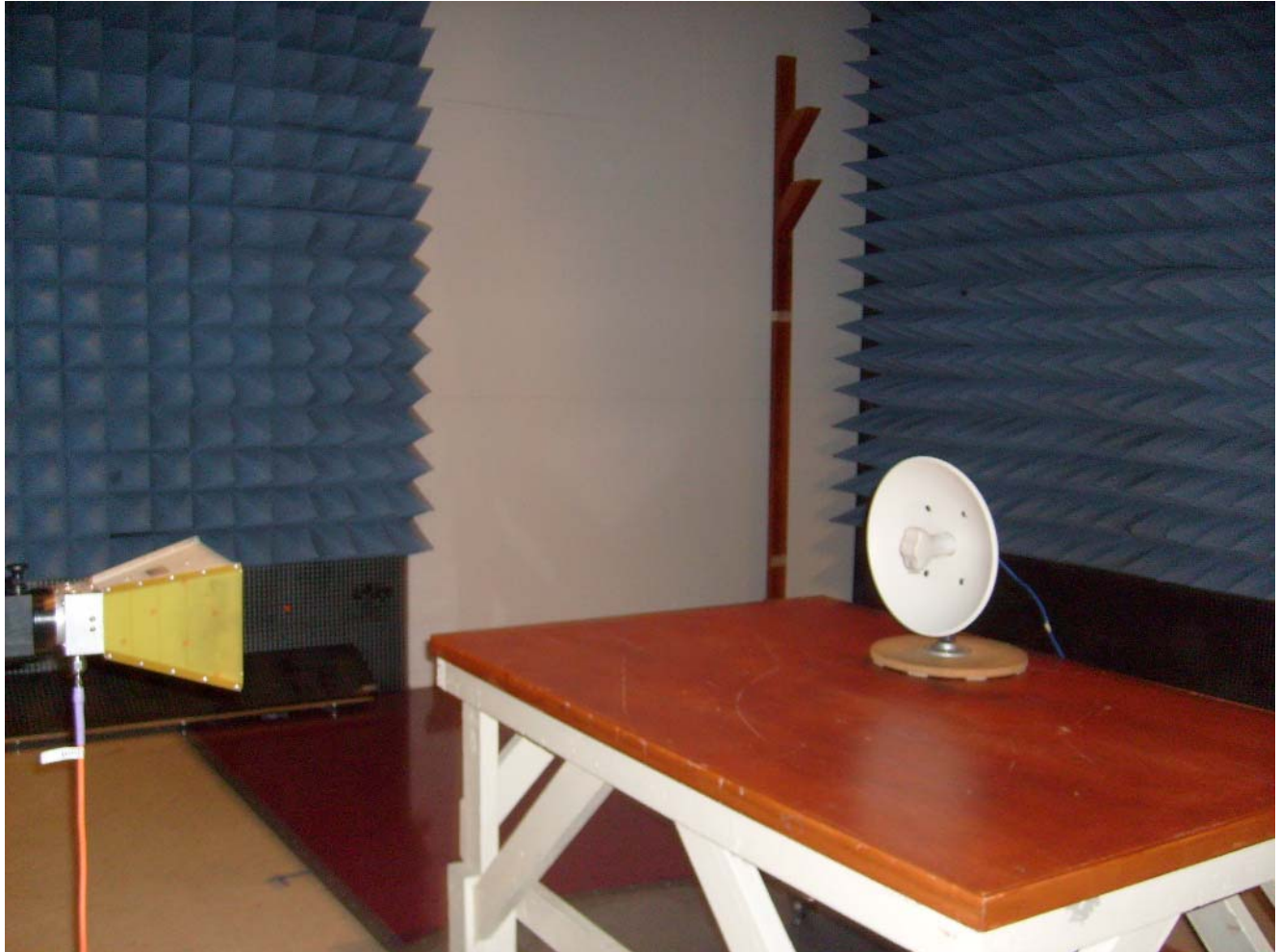
Photograph 5. Radiated Spurious, Test Setup (Dish Antenna)
