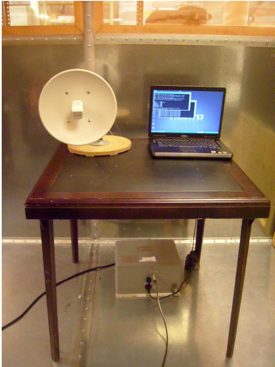
Photograph 1. Conducted Emissions, Test Setup
