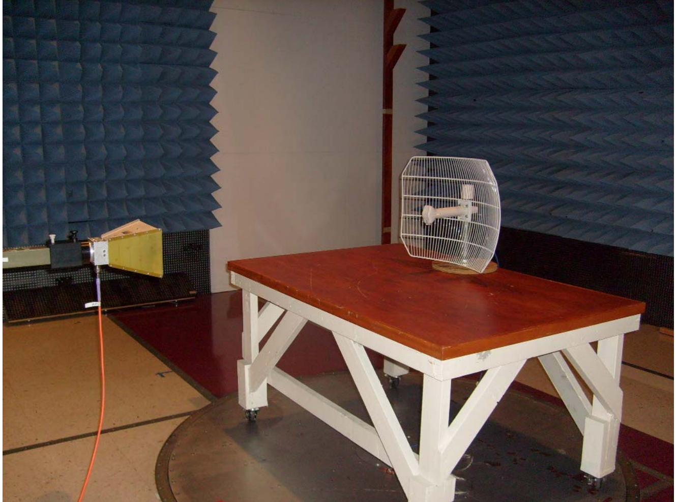
Photograph 6. Radiated Spurious, Test Setup (Grid Antenna)
