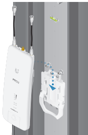
Mounting on a Sector Antenna
