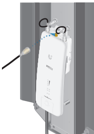
Connecting the GPS Antenna
