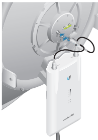
Connecting to a RocketDish
