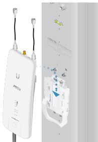
Mounting on a Sector Antenna
