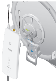
Mounting on a RocketDish
