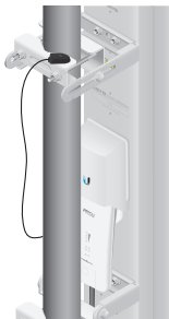
Placement on a Sector Antenna
