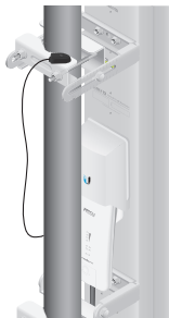
Placement on a Sector Antenna
