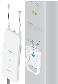
Mounting on a Sector Antenna
