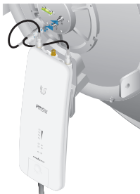
Connecting to a RocketDish
