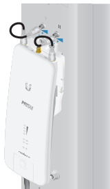
Connecting to a Sector Antenna
