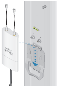
Mounting on a Sector Antenna
