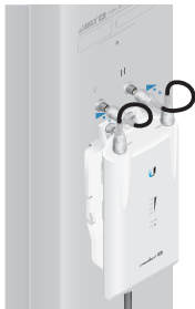
Connecting to a Sector Antenna
