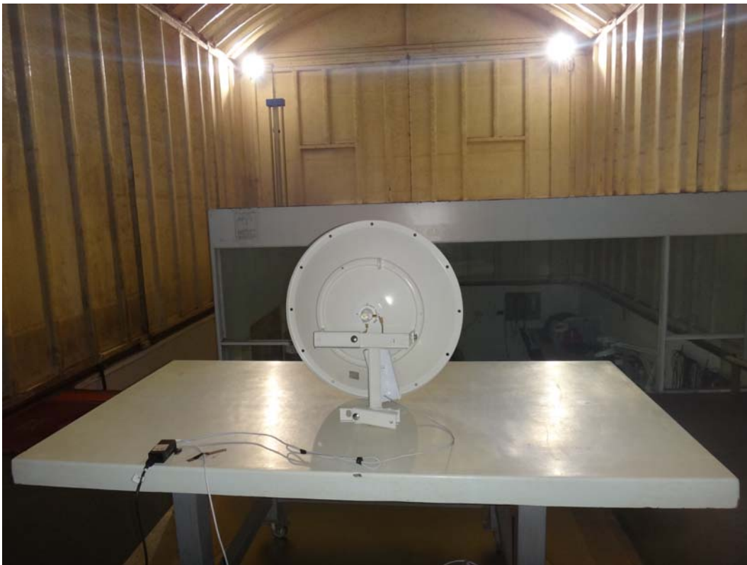
Back View of Radiated Test (Horn) - Dish Antenna
