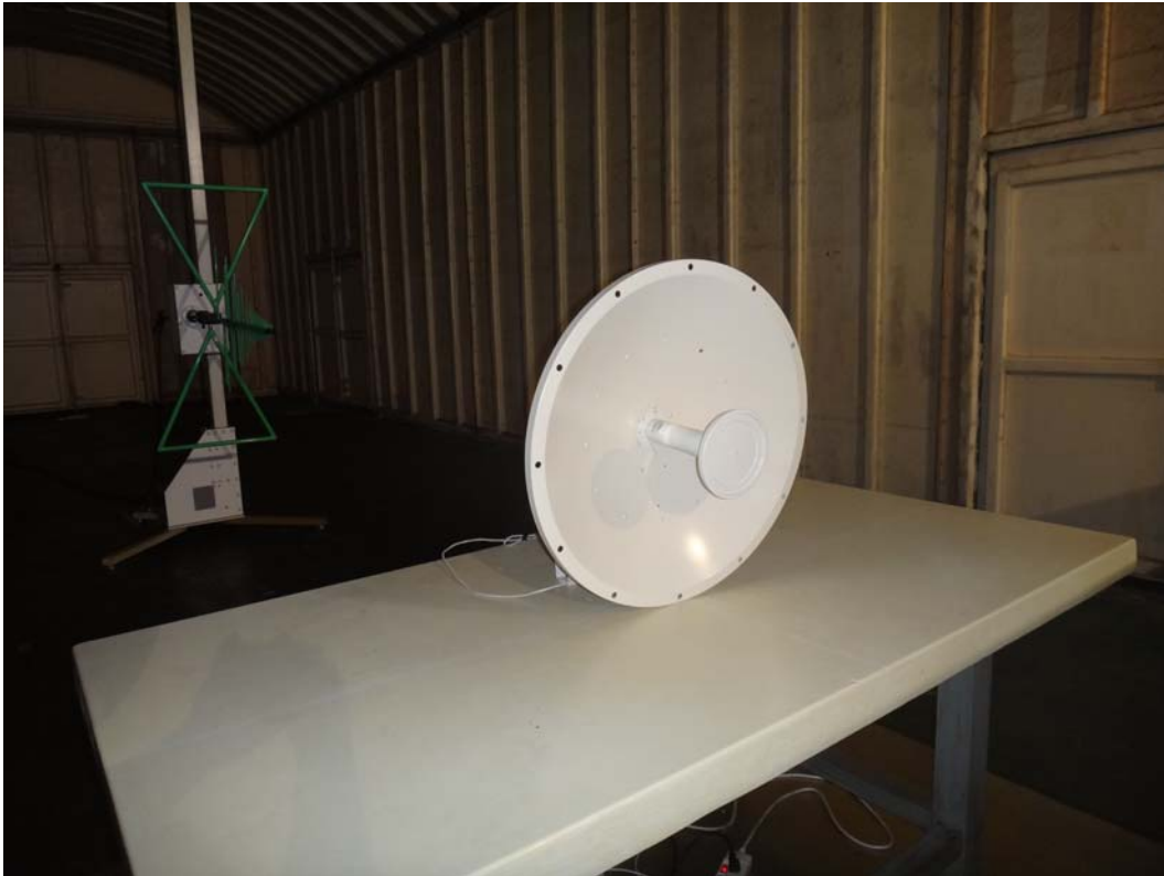
Back View of Radiated Test – Dish Antenna
