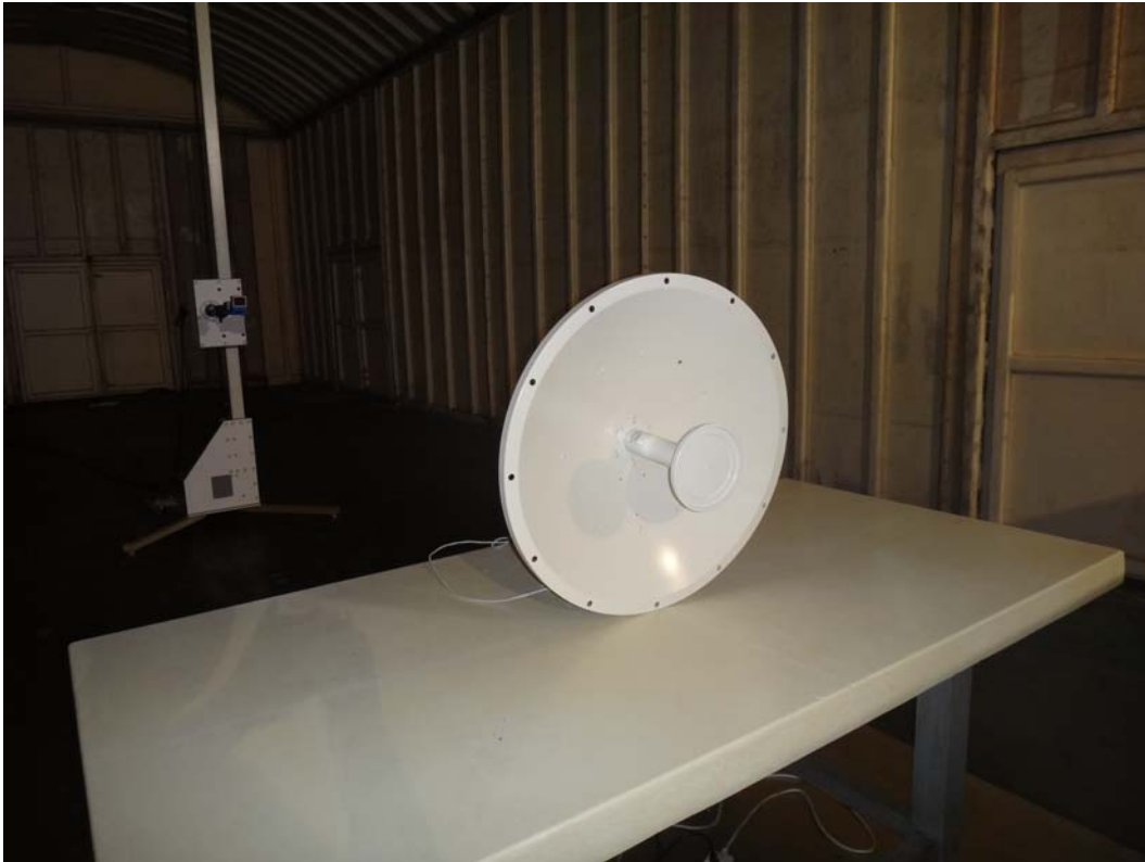
Back View of Radiated Test (Horn) - Dish Antenna
