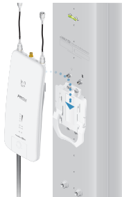
Mounting on a Sector Antenna
