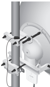
Placement on a Dish Antenna
