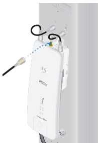
Connecting the GPS Antenna
