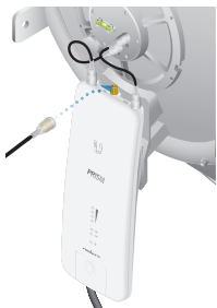
Connecting the GPS Antenna
