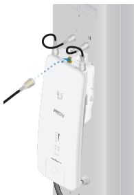
Connecting the GPS Antenna
