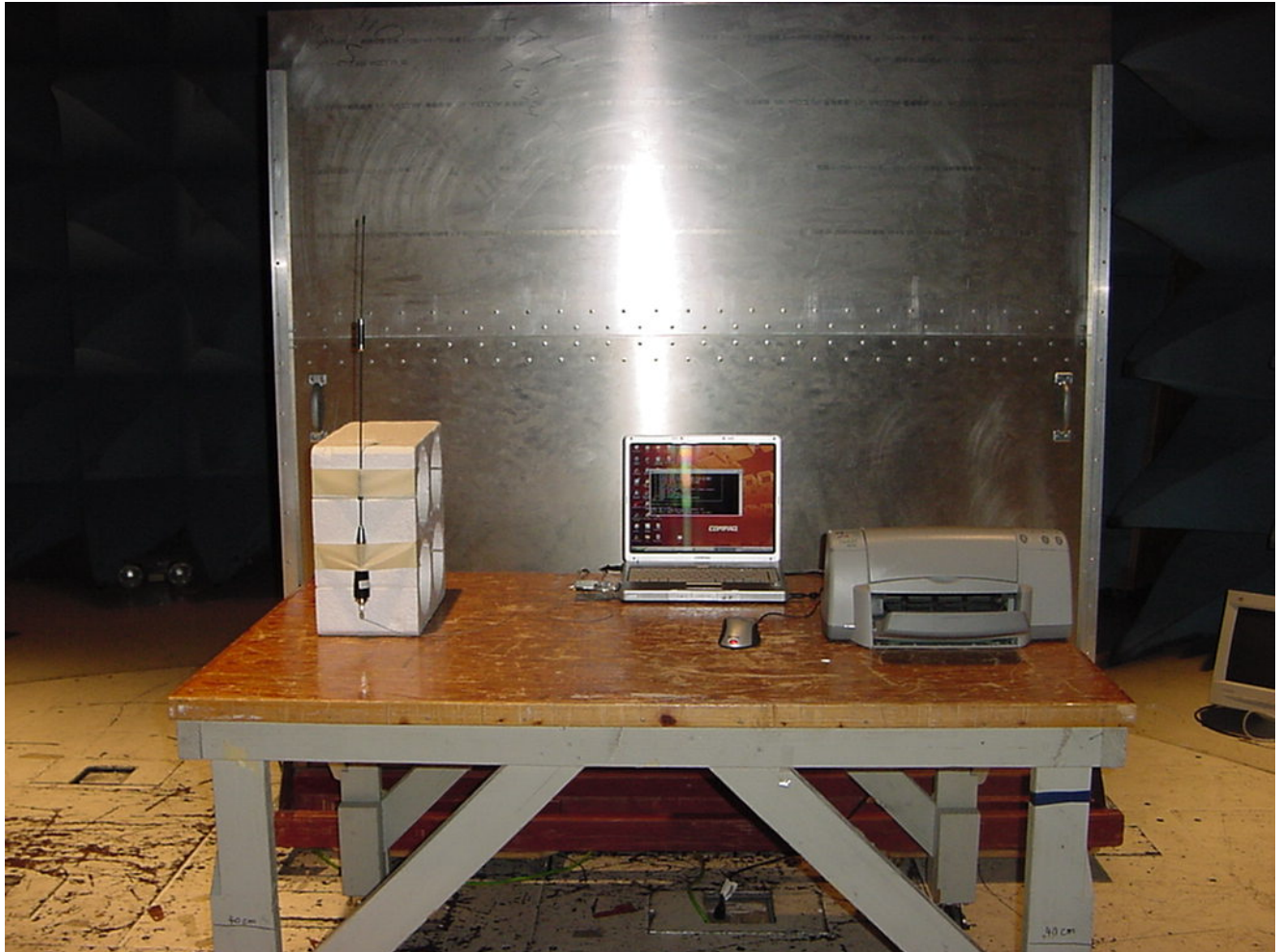
Photograph 1. Conducted Emissions Test Setup
