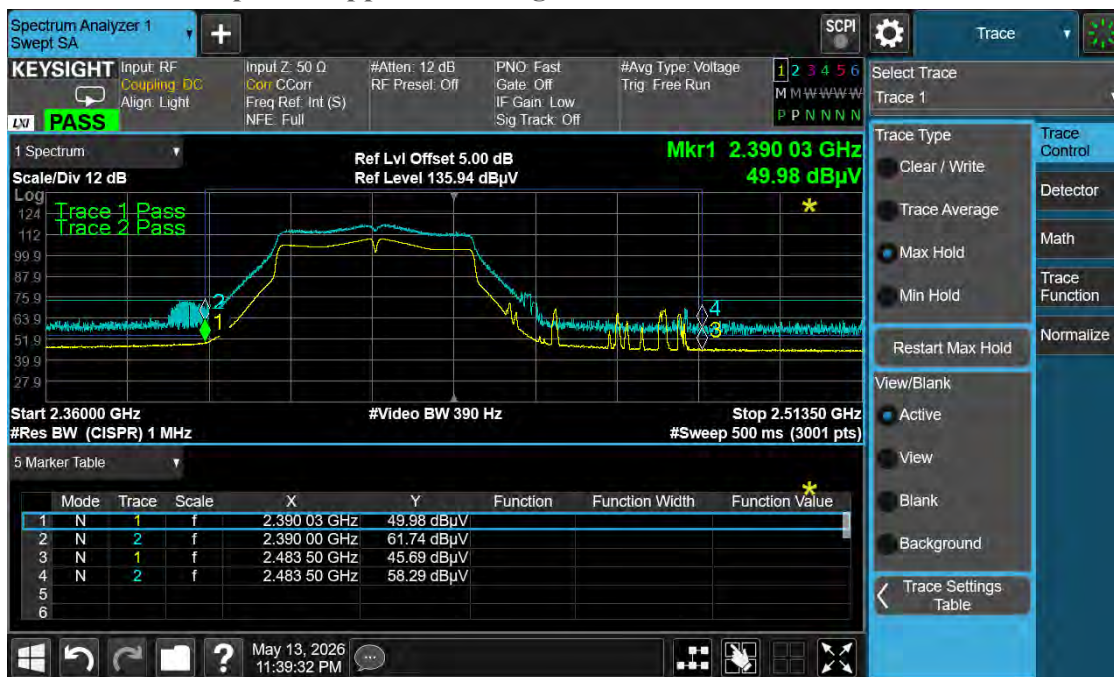
Graph 30: Lower Band Edge Plot – 2422 MHz – n40 Mode
