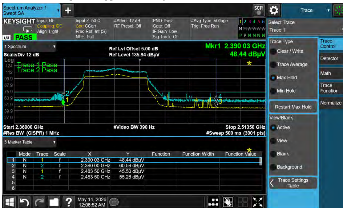
Graph 36: Lower Band Edge Plot – 2422 MHz – be40 Mode
