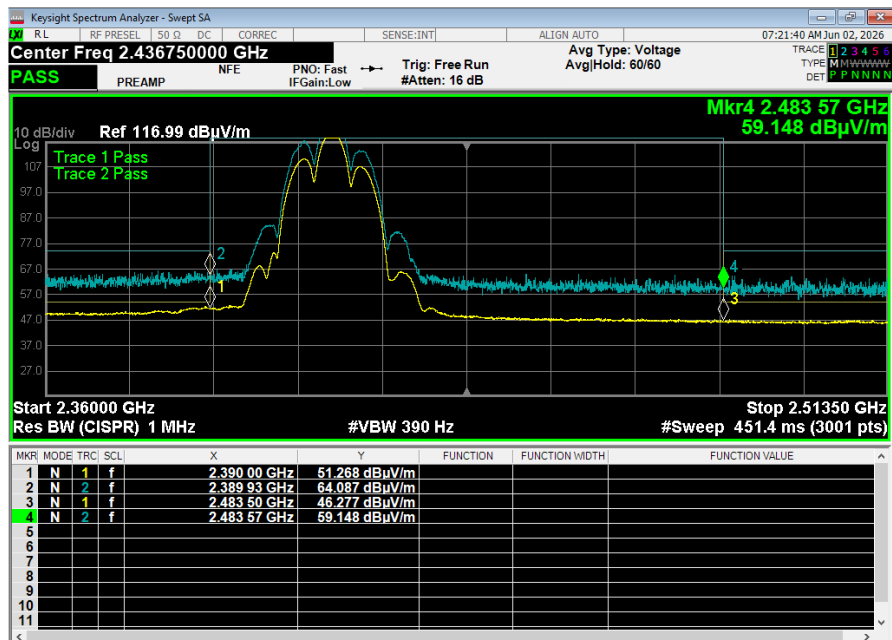
Graph 3: Lower Band Edge Plot – 2412 MHz – b Mode
