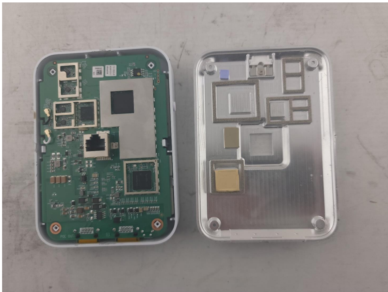
Photograph 1: Back Cover Off Showing PCB in Housing
