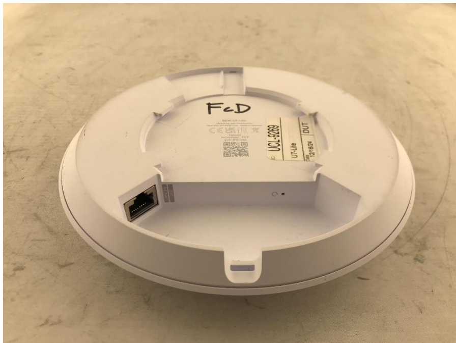
Photograph 7: Back View of DUT Showing Ethernet Port
