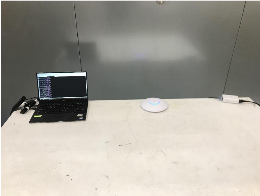
Photograph 7: View Test Set Up Front Conducted Emissions
