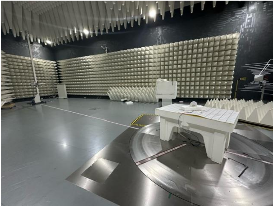
Photograph 1: View Test Set Up Radiated Emissions 30 – 1000 MHz
