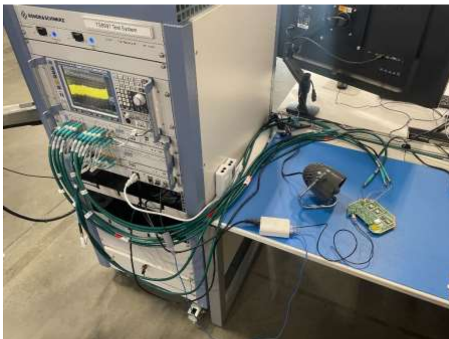
Photograph 4: View Test Set Up RF Conducted
