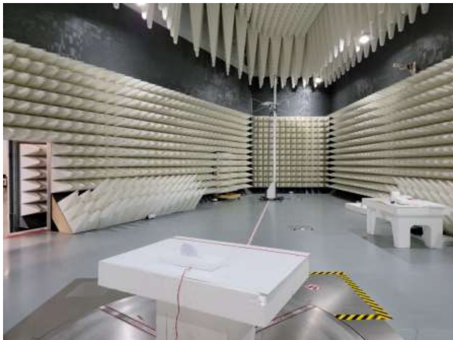
Photograph 1: View Test Set Up Radiated Emissions 30 – 1000 MHz
