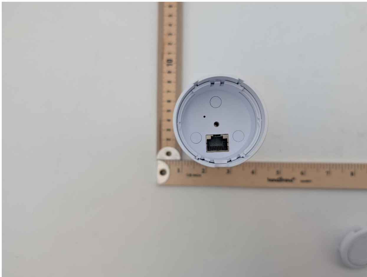
Photograph 7: Bottom View of DUT Cover Off Showing PoE Port
