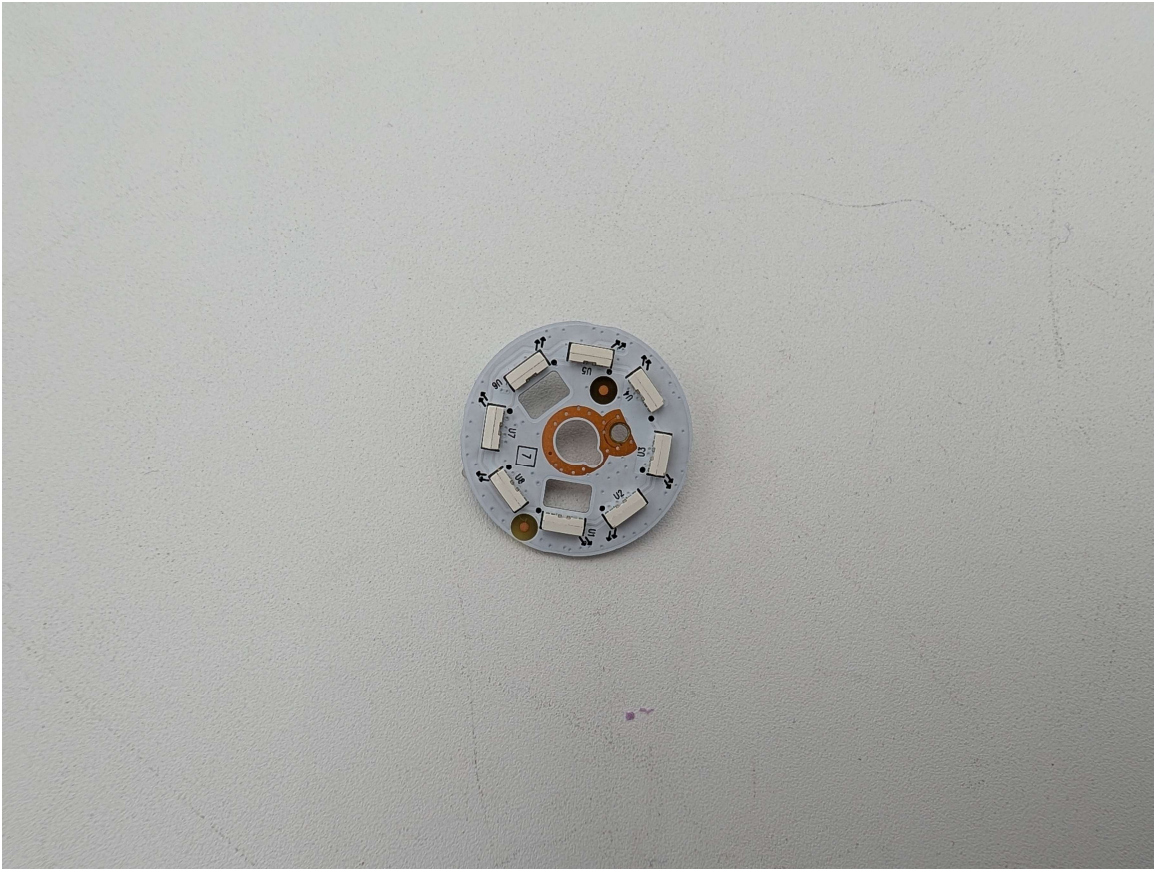
Photograph 8: Top LED PCB
