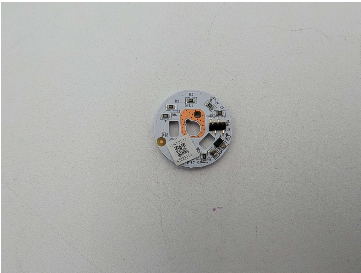
Photograph 9: Bottom LED PCB
