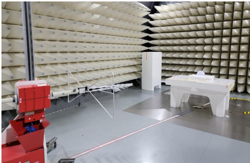
Photograph 1: View Test Set Up Radiated Emissions 30 – 1000 MHz
