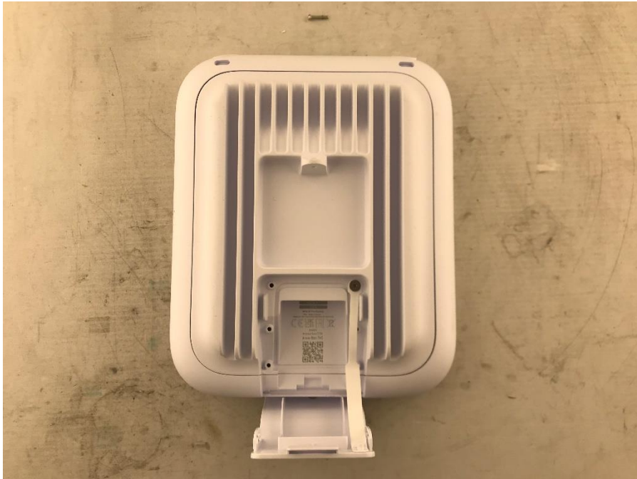
Photograph 7: Back View of DUT with Cover Removed
