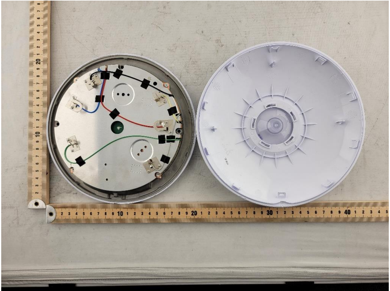
Photograph 1: Internal View of DUT Front Cover Off
