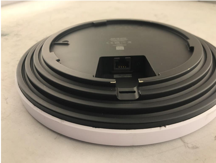
Photograph 3: Back View Close up of Ethernet Connector
