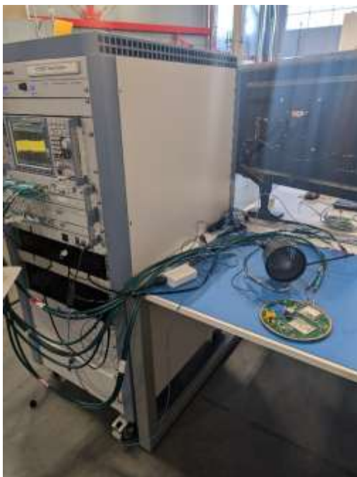
Photograph 4: View Test Set Up RF Conducted
