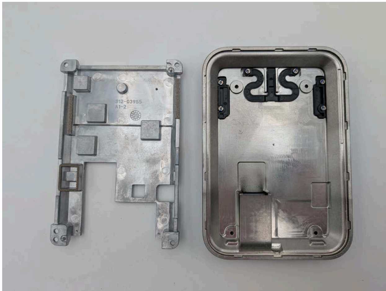
Photograph 2: Internal View Separation of Back Cover
