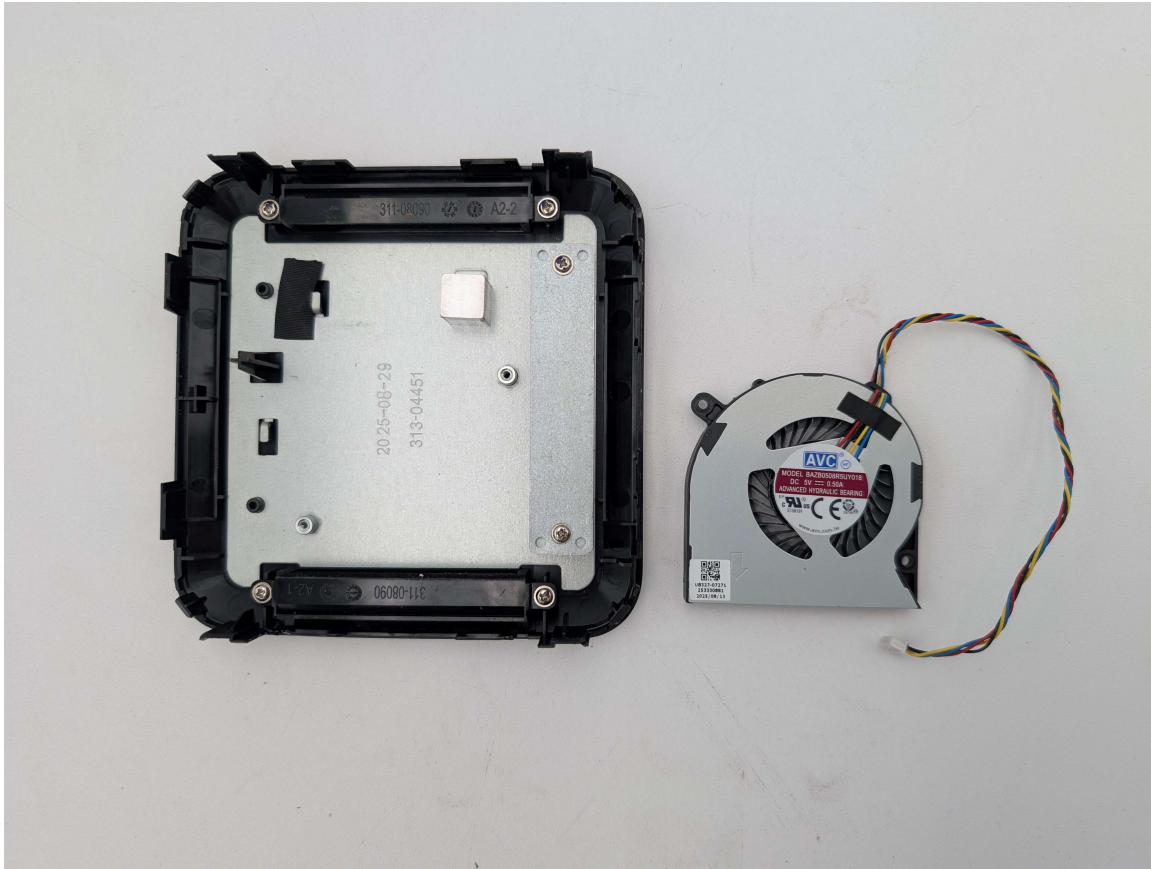
Photograph 7: Bottom Fan Housing w/ Fan Removed (Showing Back of Fan)
