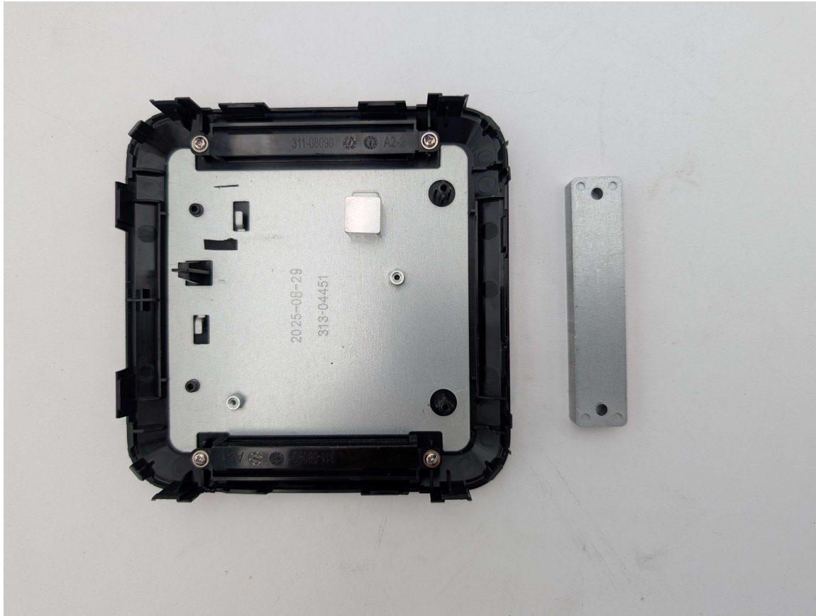
Photograph 1: Bottom Fan Housing w/ Weight Bar Removed
