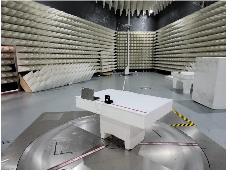
Photograph 1: View Test Set Up Radiated Emissions 30 – 1000 MHz
