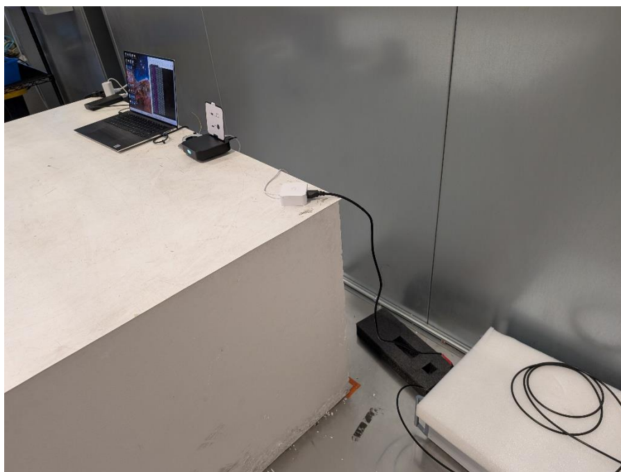
Photograph 7: View Test Set Up Front Conducted Emissions
