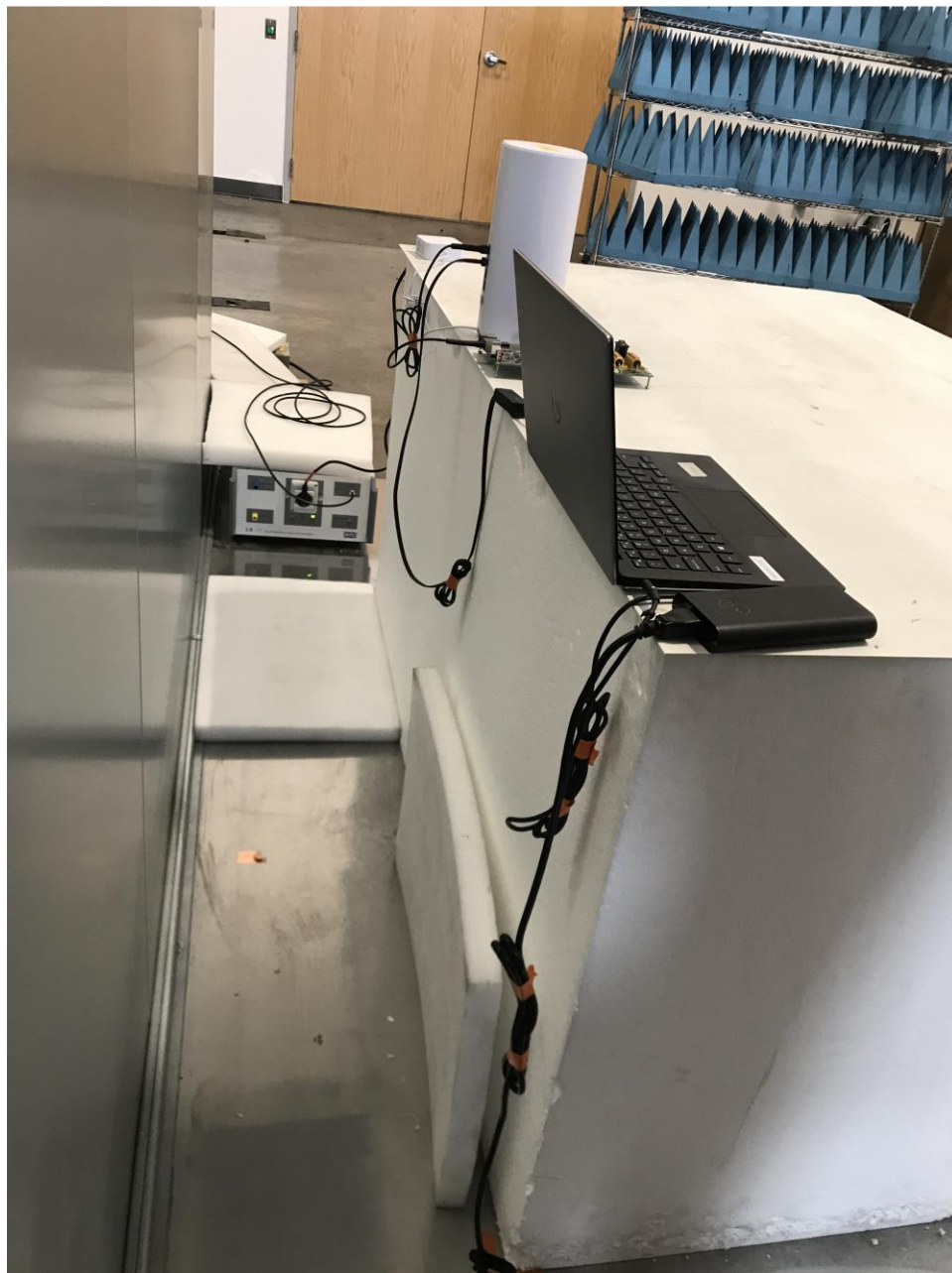
Photograph 9: View Test Set Up Back Conducted Emissions
