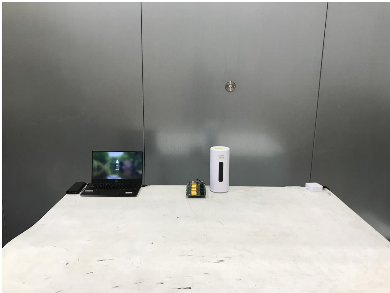
Photograph 8: View Test Set Up Front Conducted Emissions
