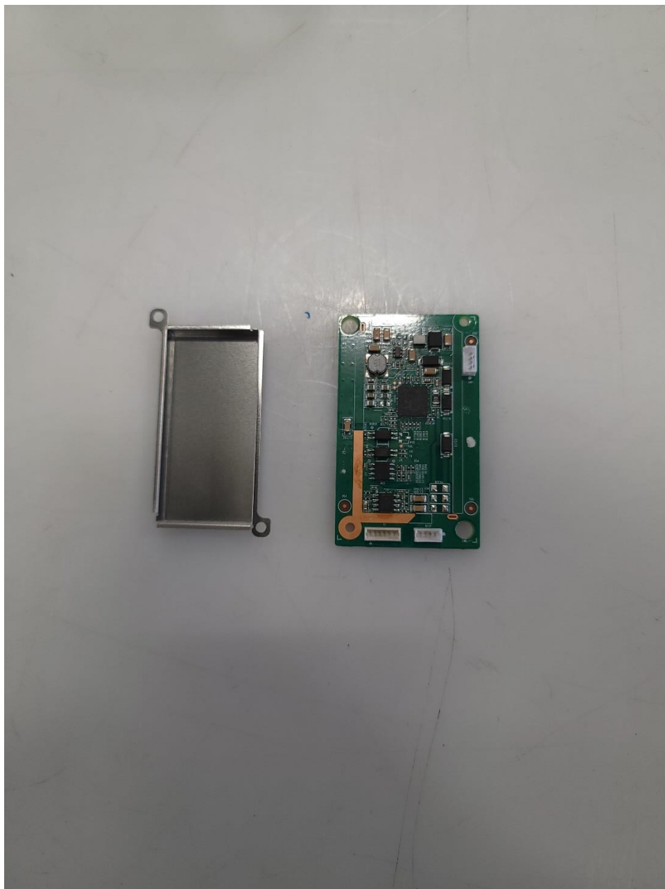
Photograph 12: Power Control Board Front
