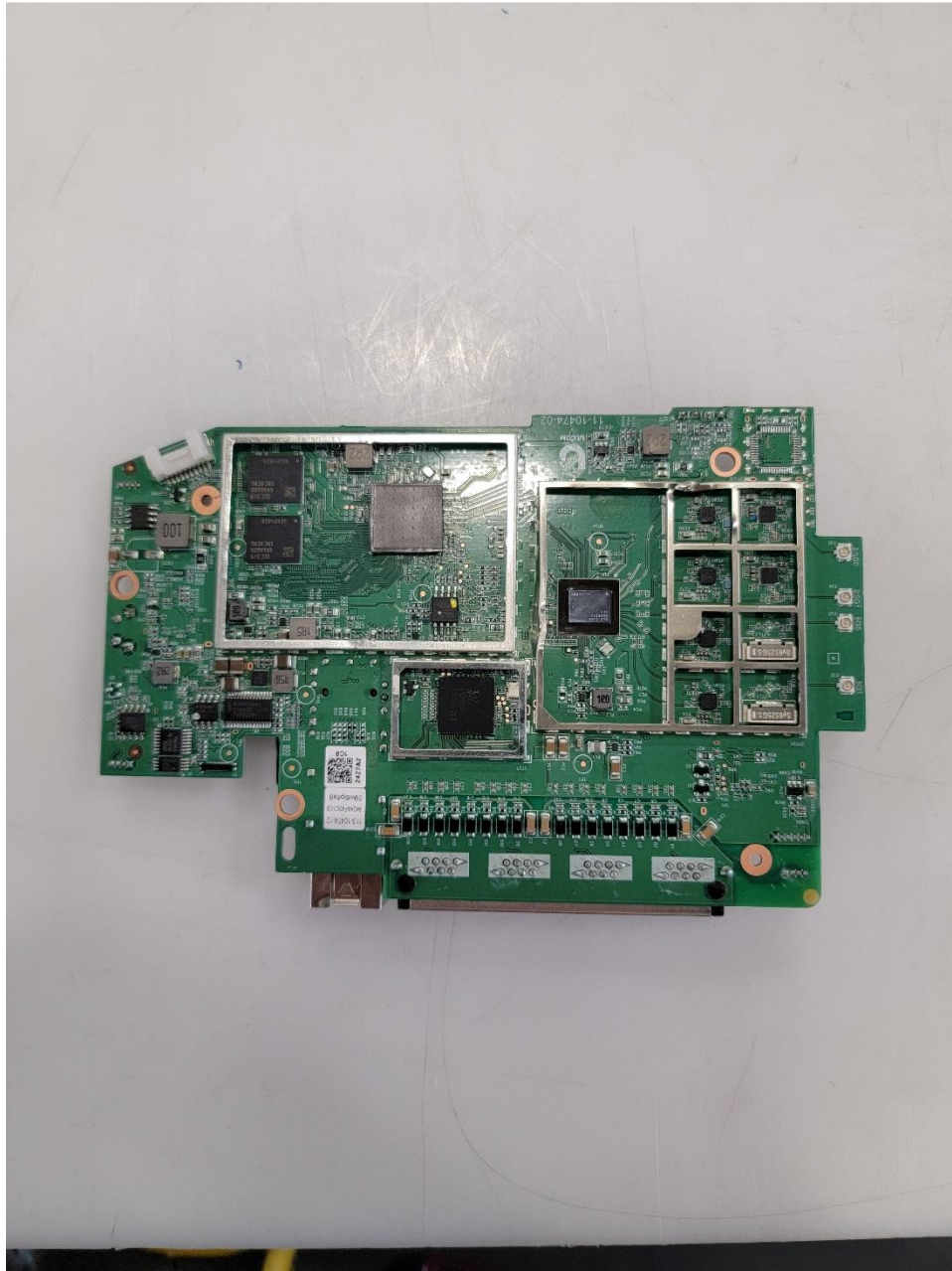
Photograph 21: Main PCB Back w/Cans Off
