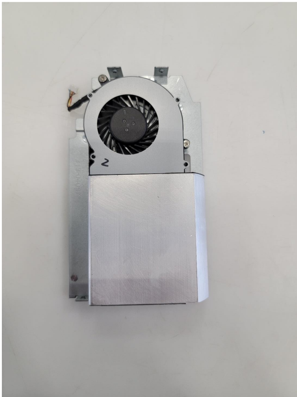
Photograph 28: Fan & Heat Sink Front
