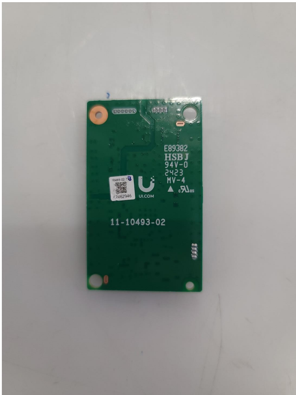
Photograph 13: Power Control Board Back
