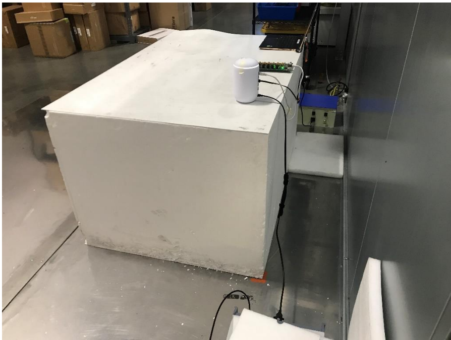
Photograph 6: View Test Set Up Back Conducted Emissions
