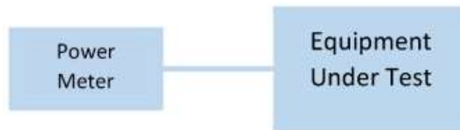
Figure 3: Output Power Measurement
