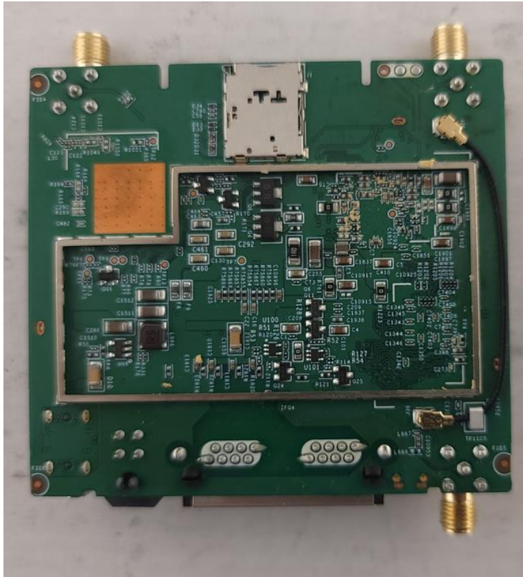
Photograph 6: Internal View of DUT – Bottom of PCB With Metal and Cans Off
