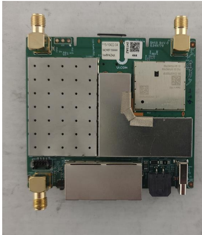
Photograph 3: Internal View of DUT – Top of PCB With Cans On
