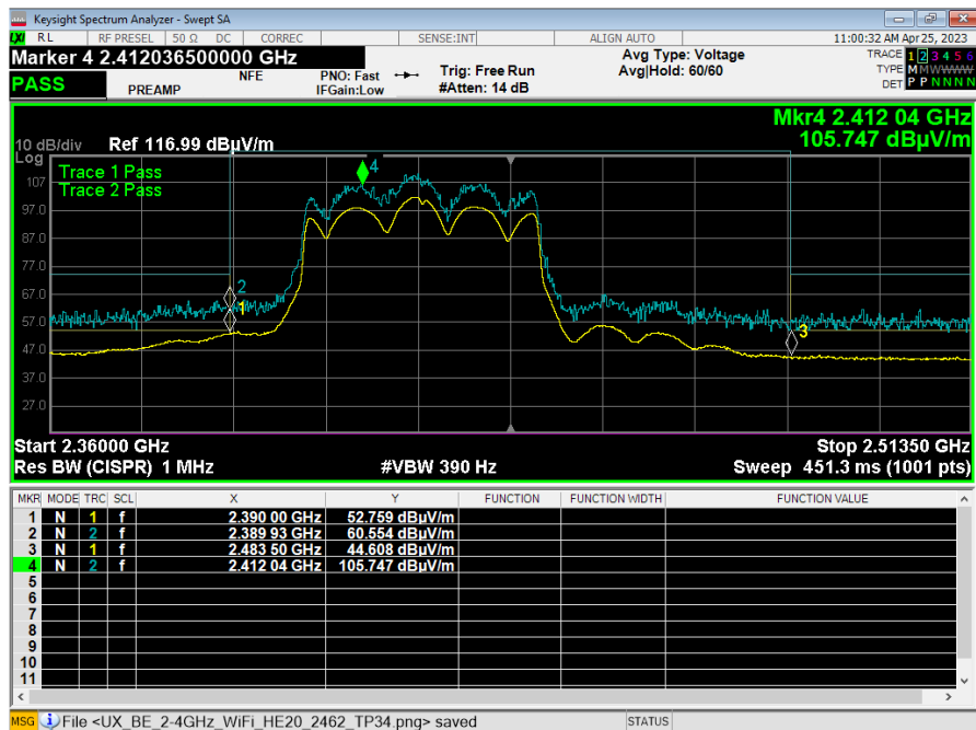
Graph 29: AX- Mode 40MHz Lower Band Edge Plot
