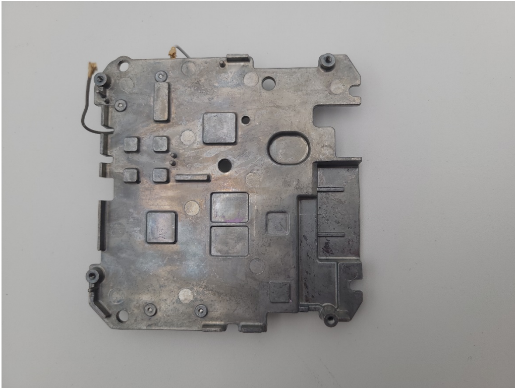
Photograph 8: Antenna Mount Bottom
