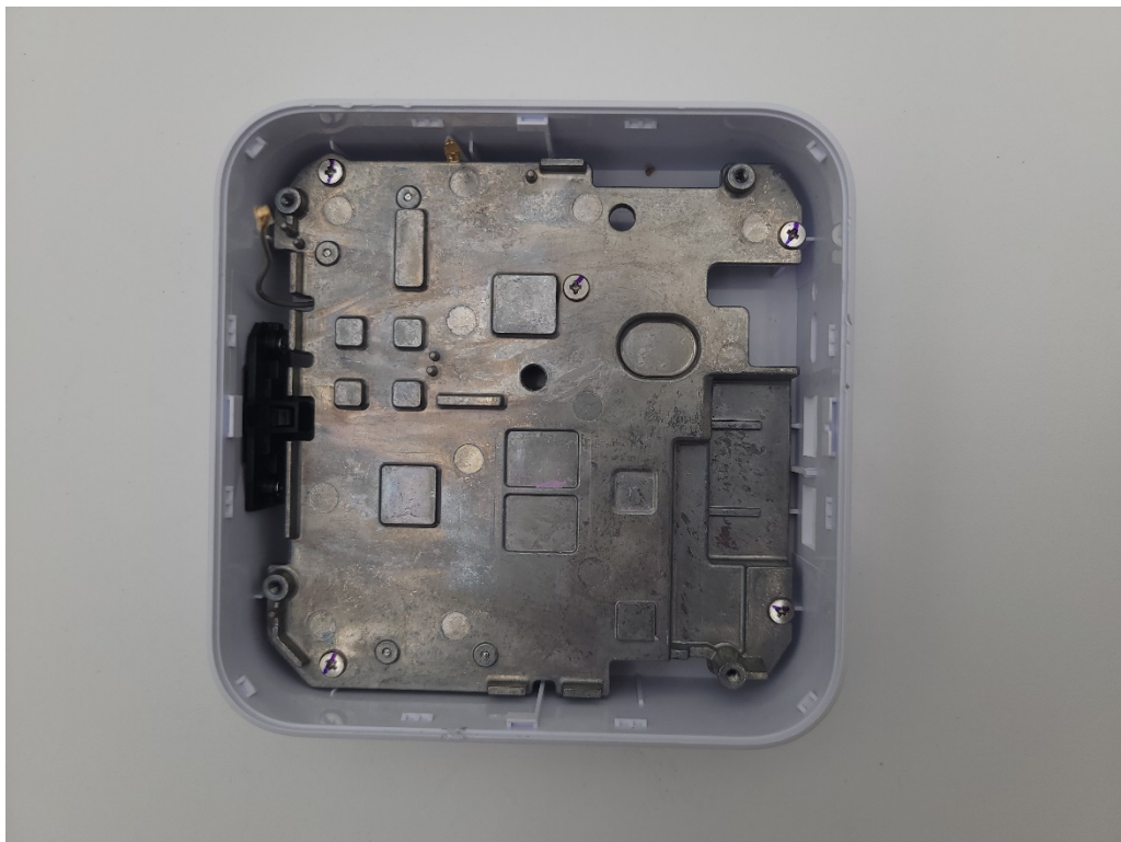
Photograph 6: Antenna Mount in Top of DUT
