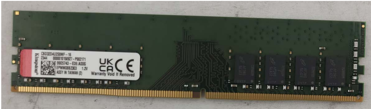
Photograph 2: Top PCB of Memory Card
