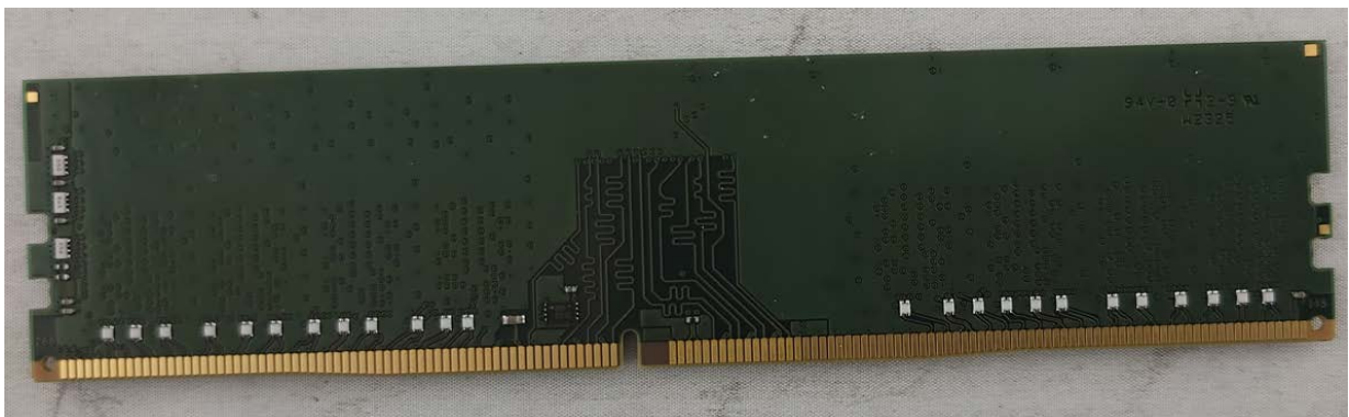
Photograph 3: Bottom PCB of Memory Card
