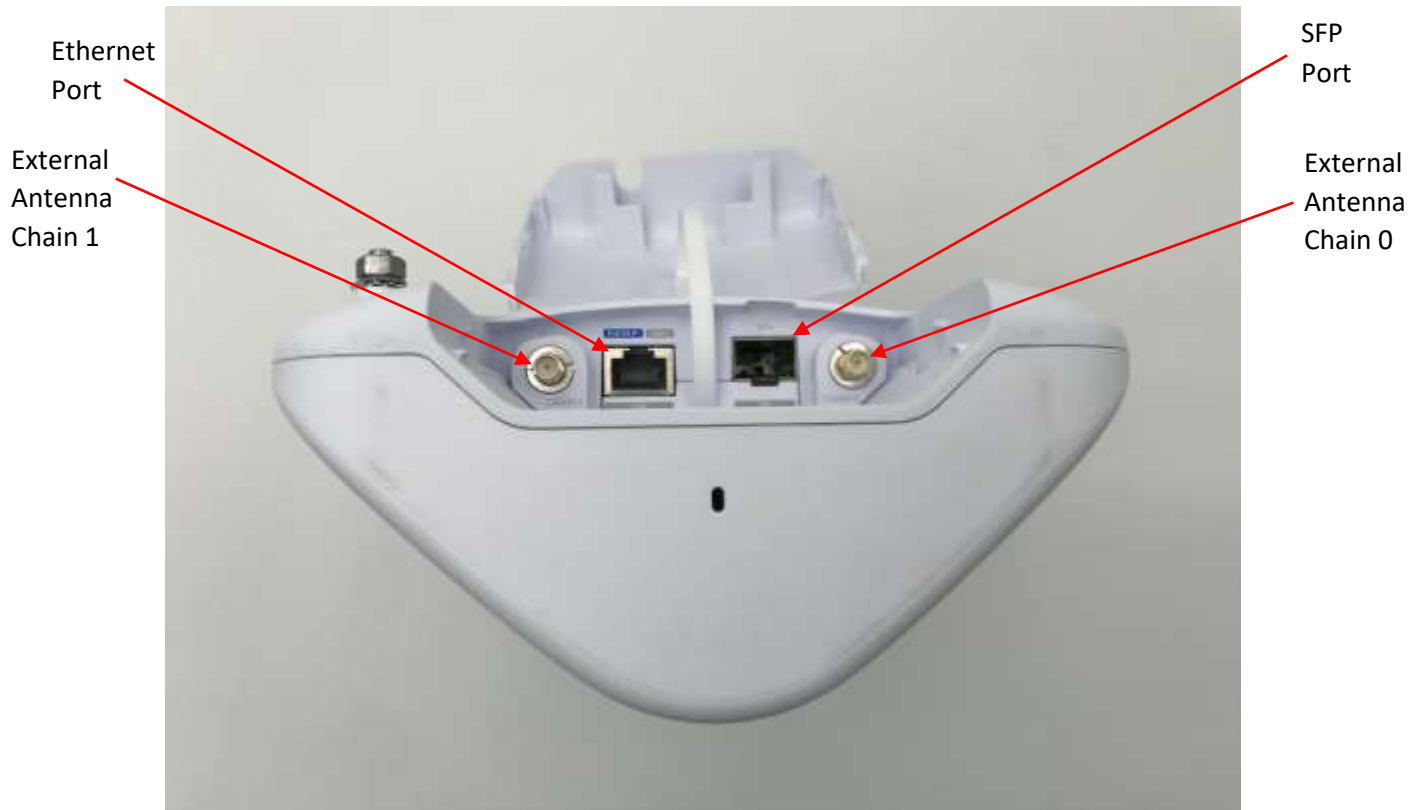
Photograph 7: Bottom Close-up of Connectors
