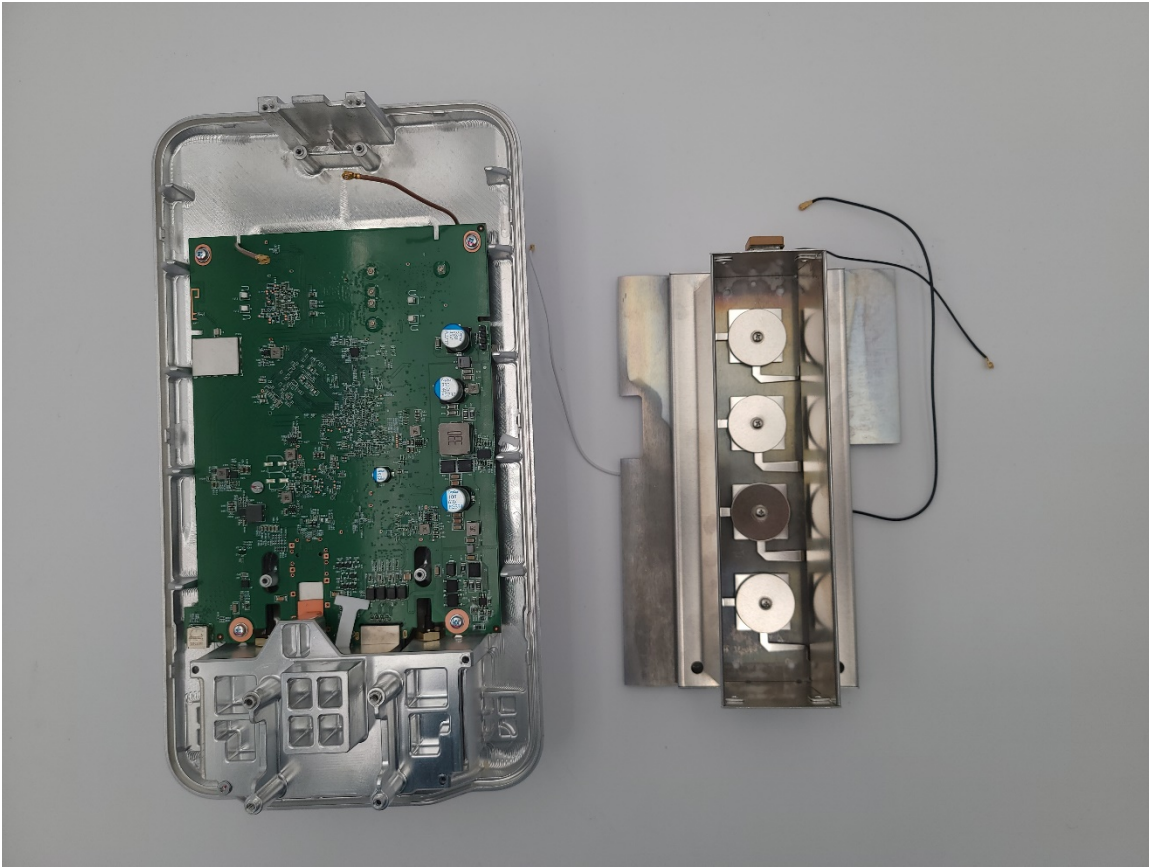
Photograph 5: 5 GHz Transmitter Board Removed
