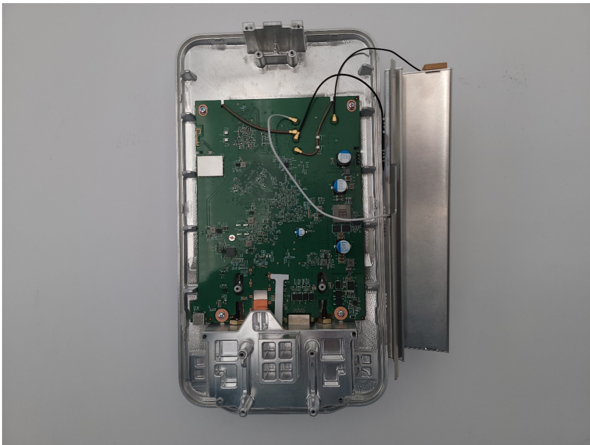
Photograph 4: 5 GHz Antenna Board Removed
