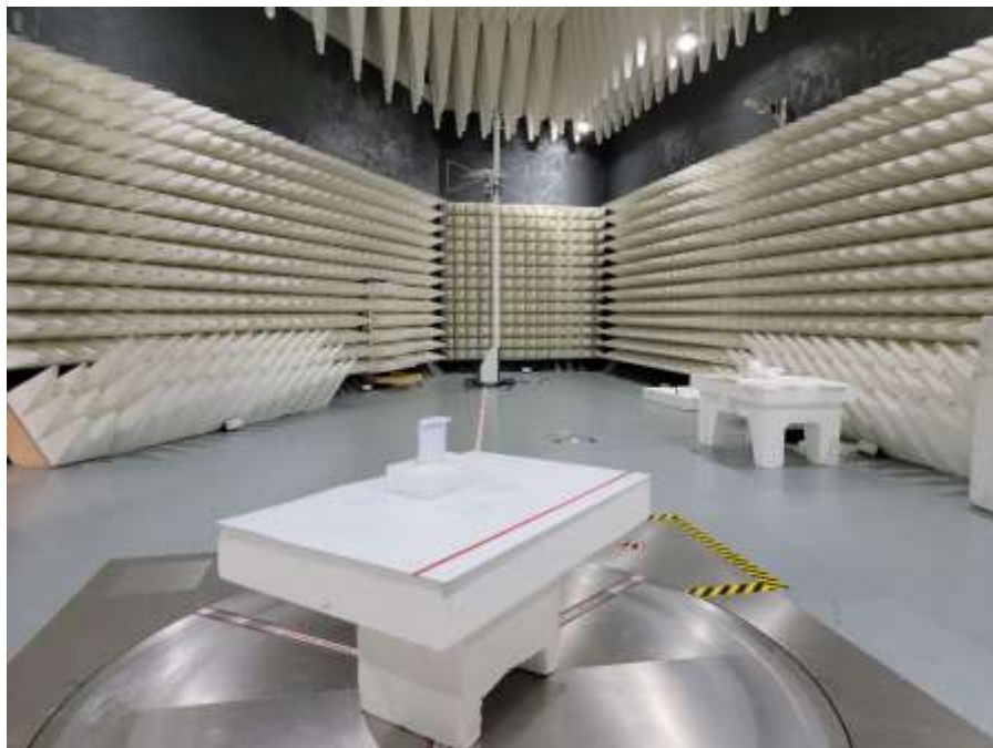
Photograph 1: View Test Set Up Radiated Emissions 30 – 1000 MHz
