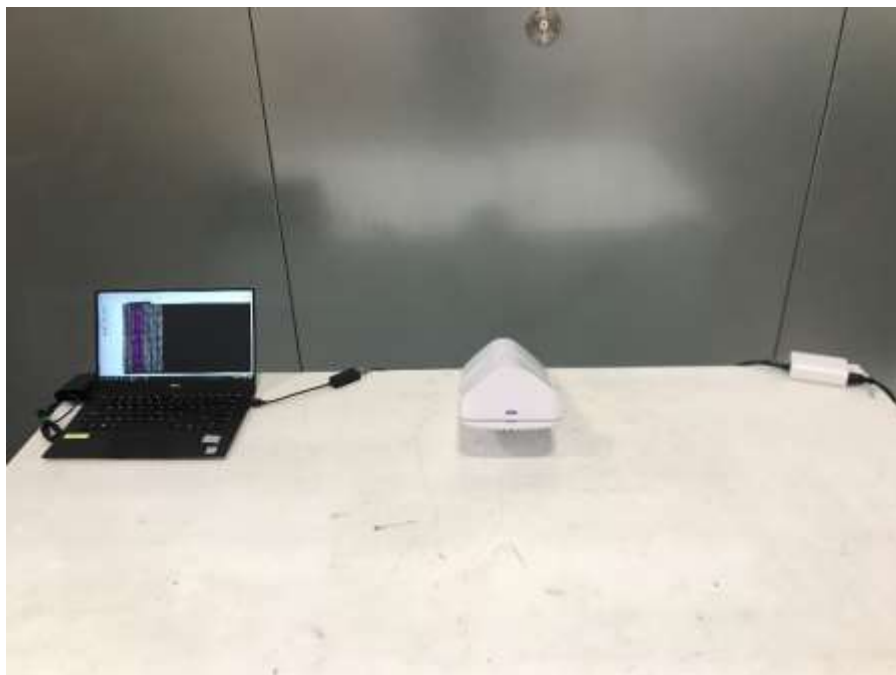
Photograph 6: View Test Set Up Front Conducted Emissions
