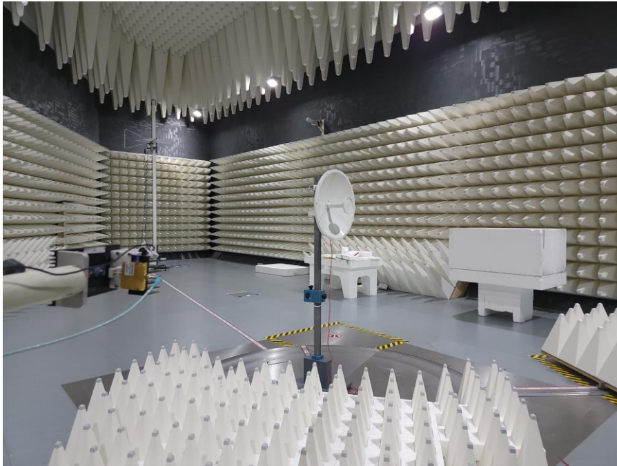
Photograph 3: View Test Set Up Radiated Emissions 17 – 40 GHz
